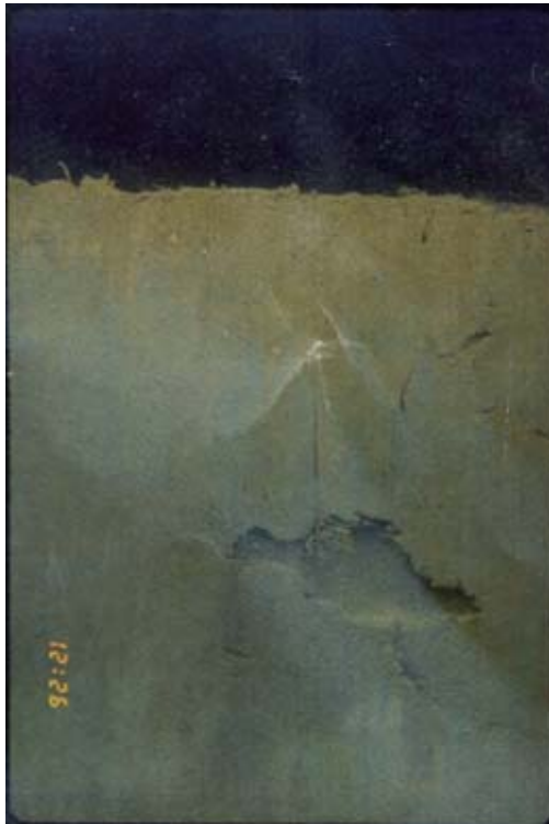
Figure 12. Example Sediment Profile Image (approx. 15x30 cm cross section). Hi-resolution photos of the upper several cm of sediment can identify a number of important parameters not easily assessed with traditional acoustic bottom mapping techniques. These include thickness of newly deposited dredged material, depth to redox discontinuity, grain size and texture, and the successional “stage” of the benthic infaunal community. This image of an undisturbed bottom shows no dredged material deposit, and the presence of a “stage 3” community as indicated by the large feeding void.
