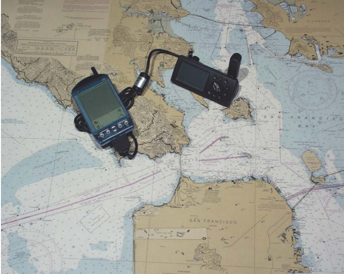
Figure 7. ADISSPalm hardware consists of a Palmtop Visor™ interfaced to a portable GPS receiver.
