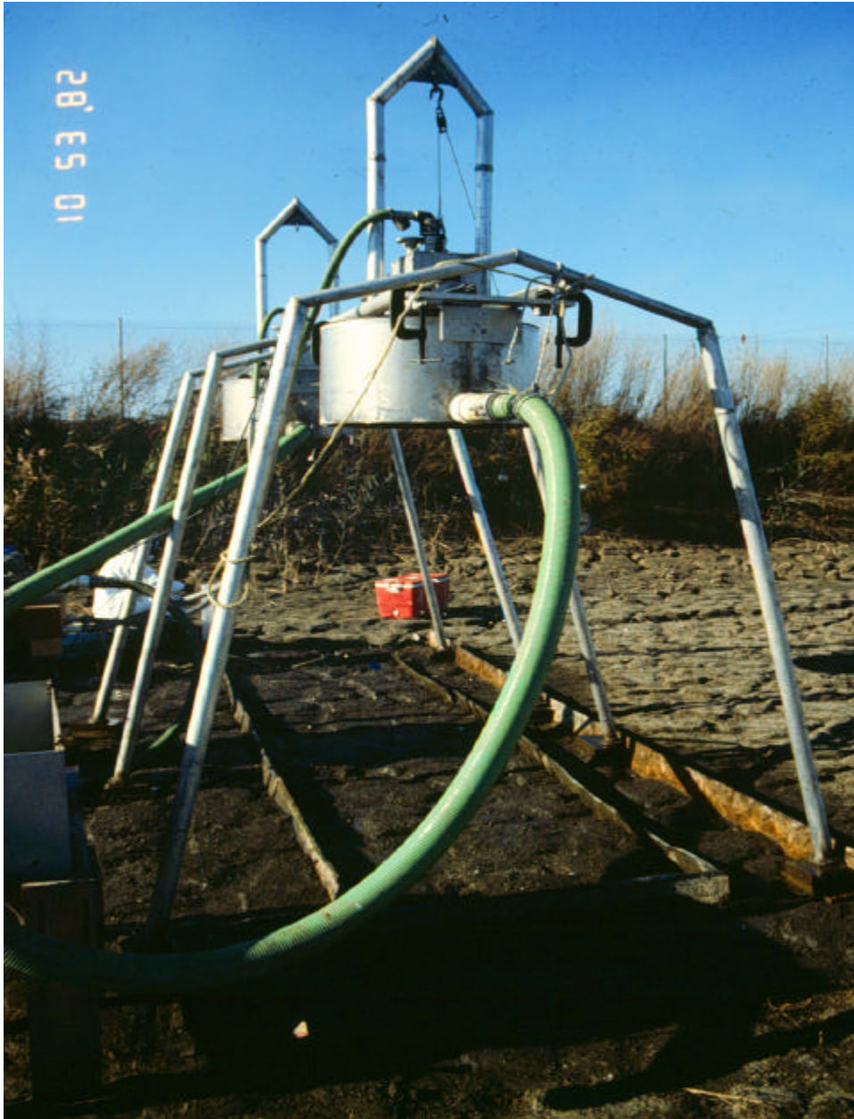
Figure 5-4. Photo of the Rainfall Simulator/Lysimeter System (RSLs)
