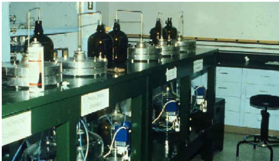
Figure 6-5. Photo of Pancake Column Leach Test setup
