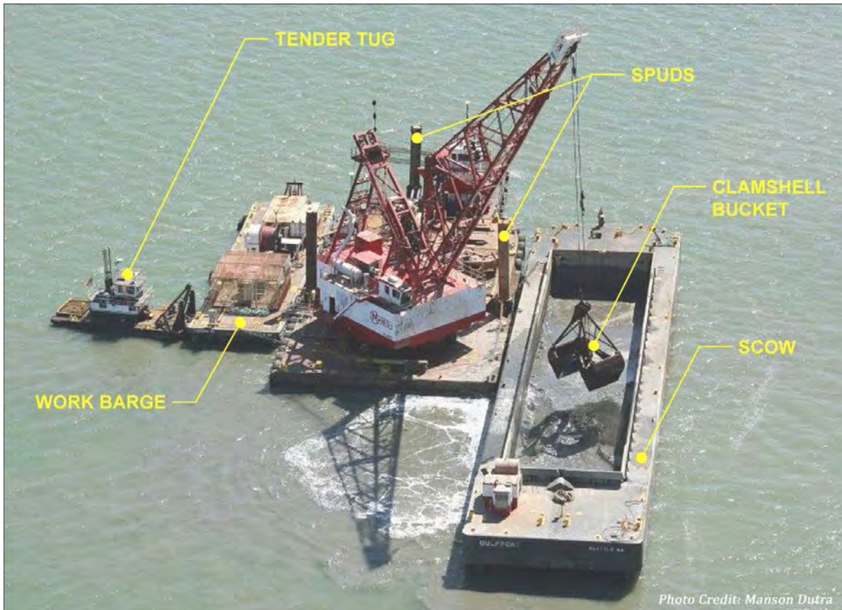
Figure 19. Typical Clamshell Dredge Plant with Scow and Tugboat.
