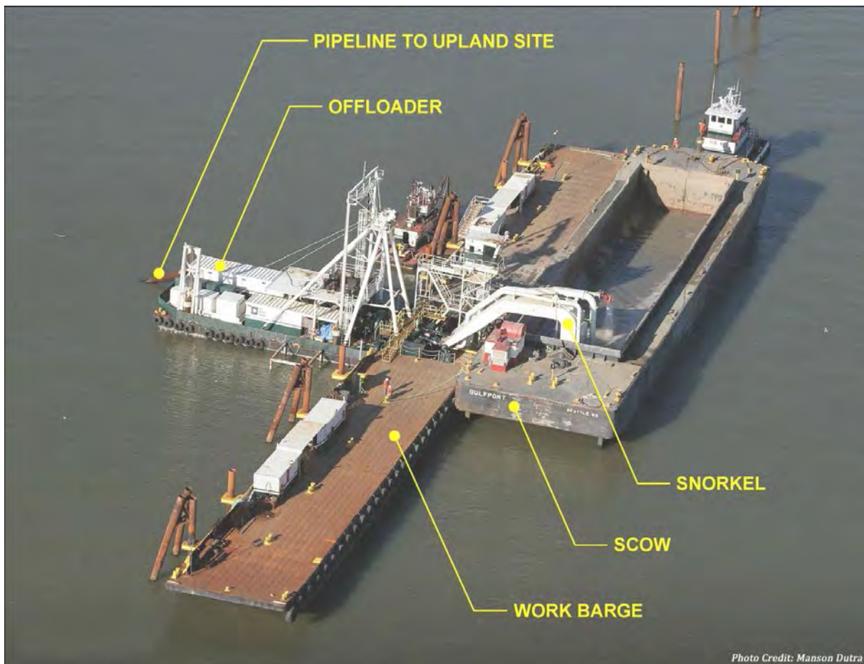
Figure 10- Offloader Liberty Unloading a Scow
