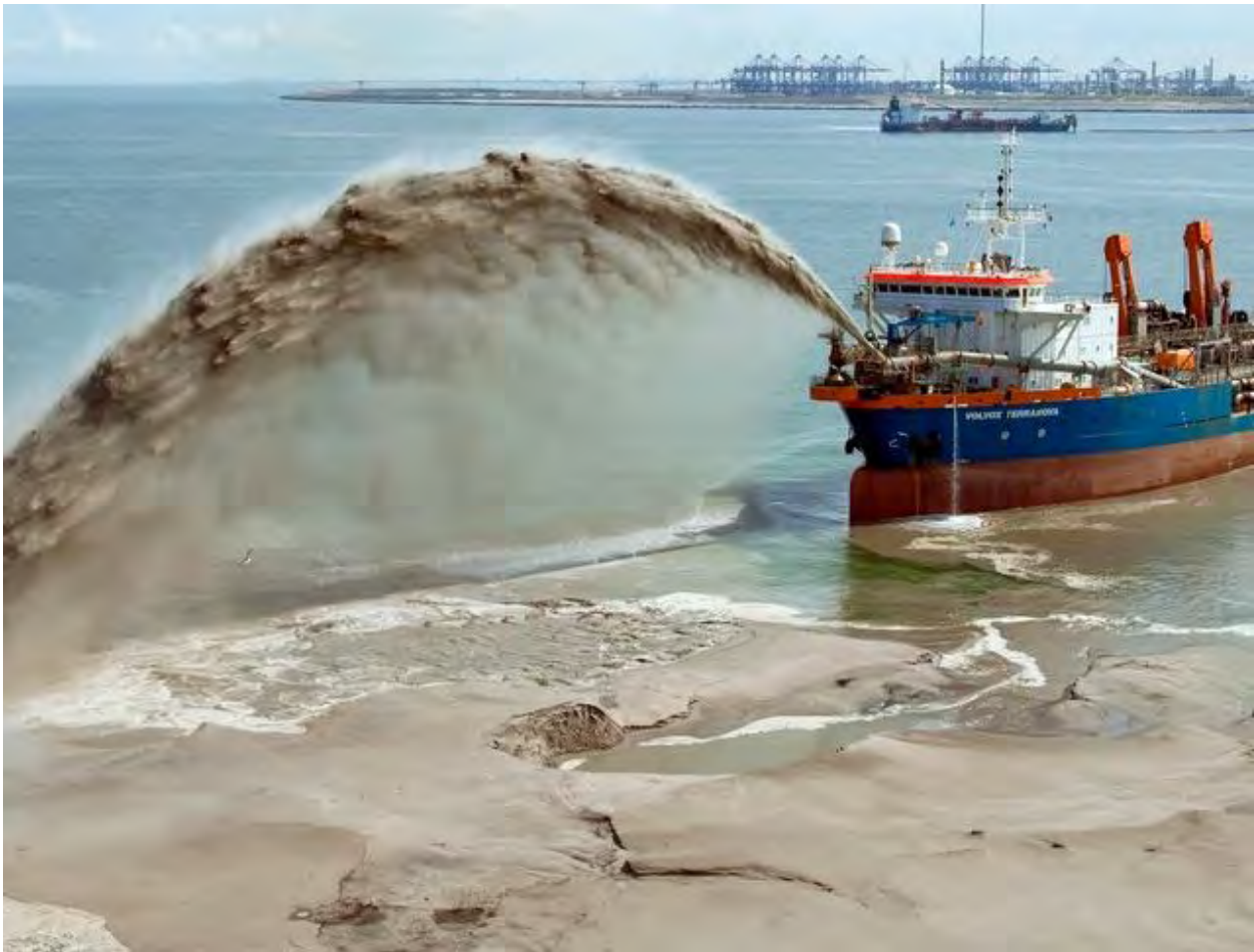
Figure 8- Hopper Dredge with Pump-Off Capability
