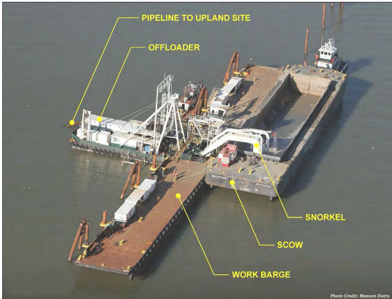
Figure 21. Liberty Offloader Unloading a Scow.
