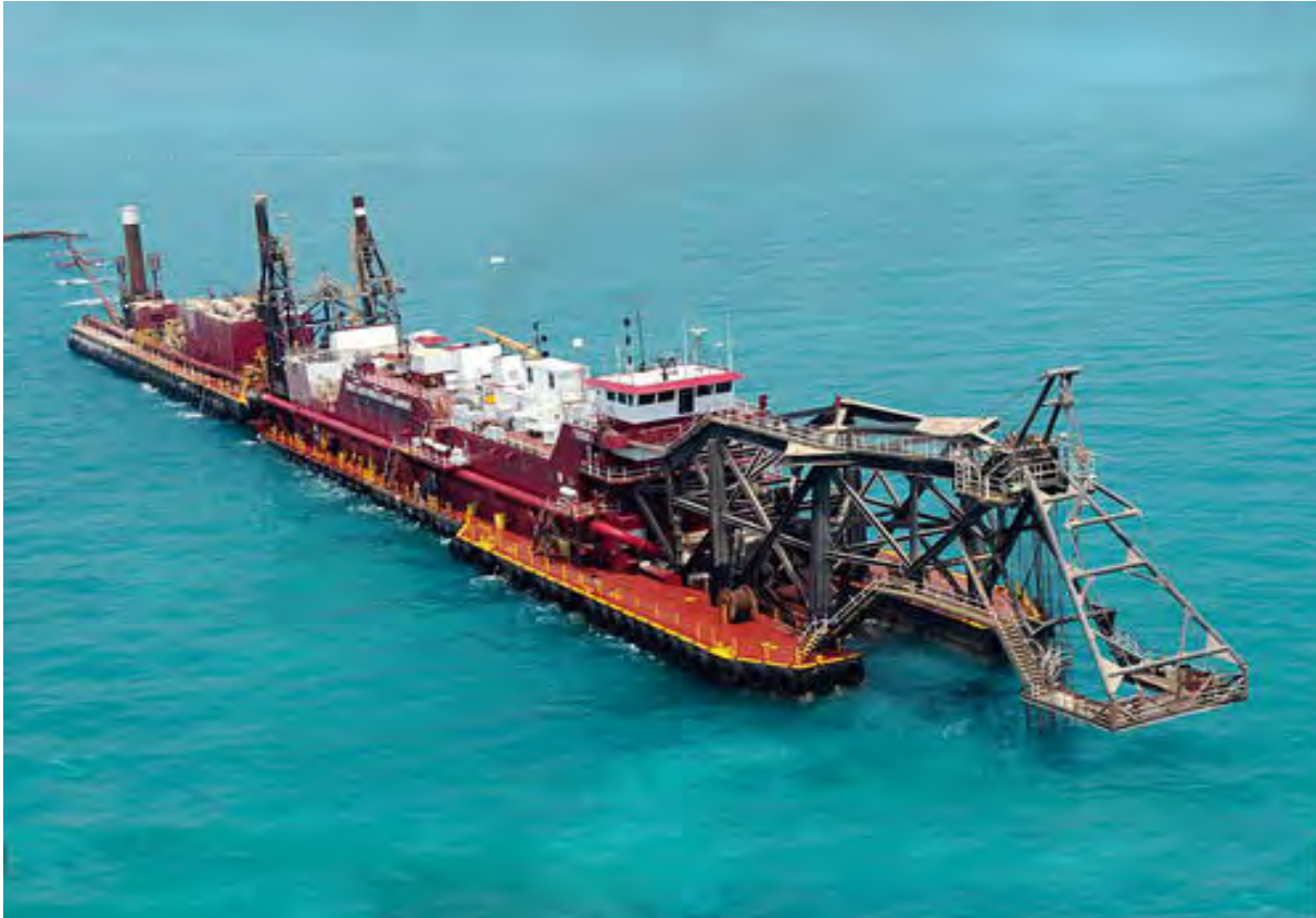
Figure 5- Typical Hydraulic Cutterhead Dredge Plant
