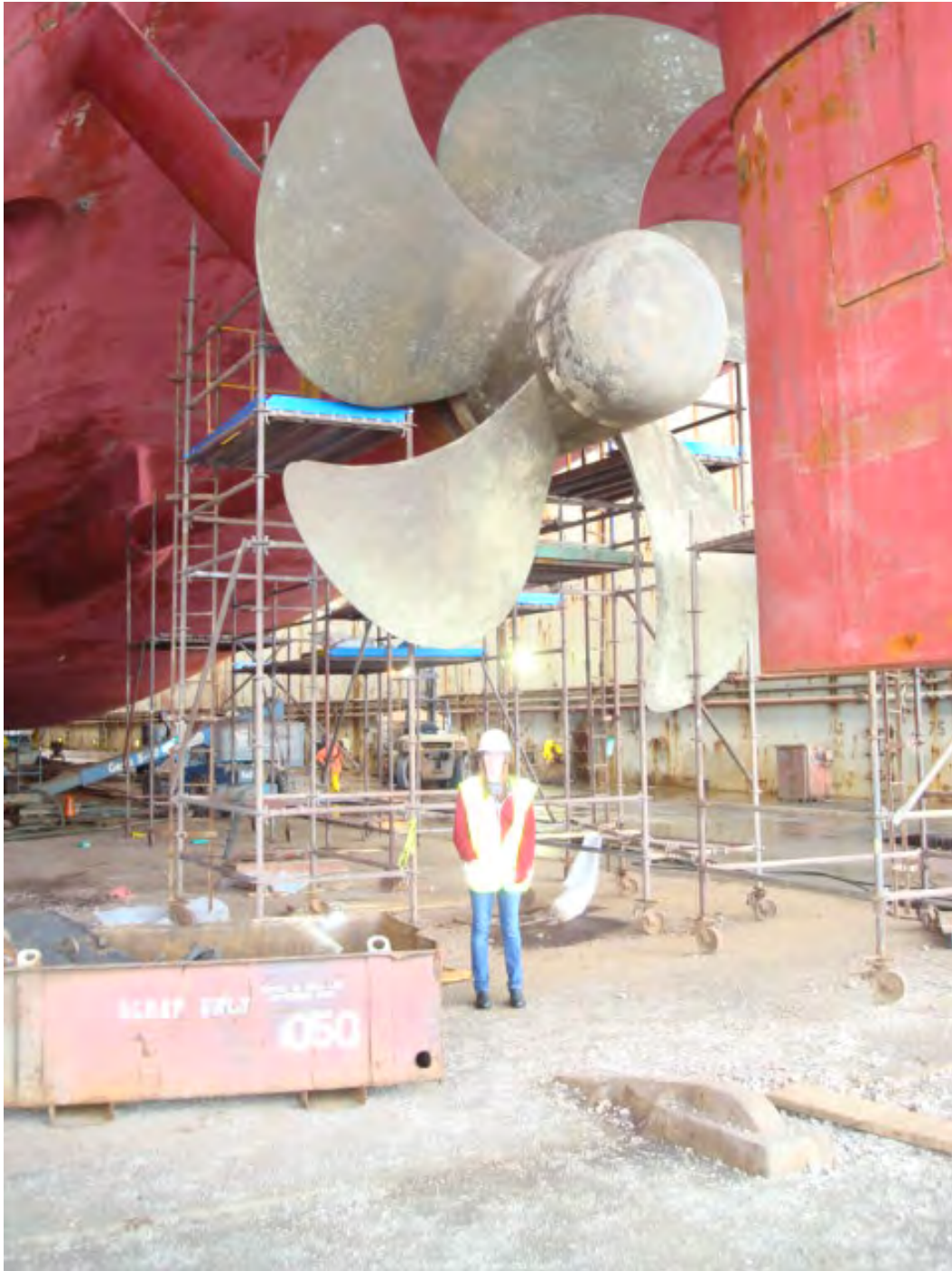
Figure 4. A ship in drydock, on reinforced pilings for hull maintenance and repairs.
