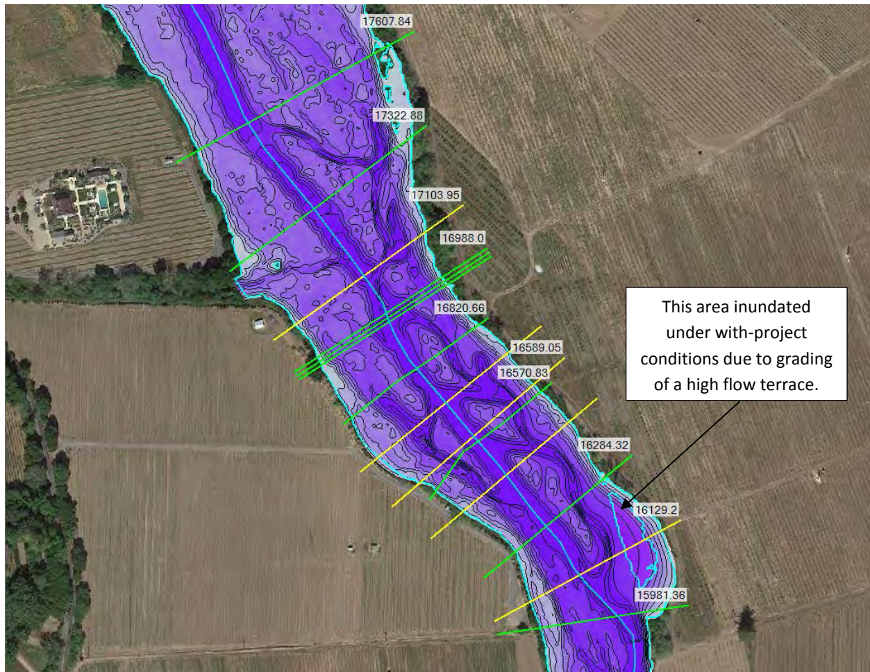
Figure 11. Water depths and flood inundation extents for the 100-year event along subreach 4A. Legend – Light Blue Outline = FWOP conditions, Deep Purple Fill = With-project conditions.
