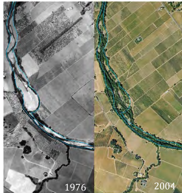
Figure 3. Example of vegetative establishment in relatively wider area of channel corridor leading to a narrowed active channel near the confluence of Grape Creek (river mile 7.3). Grape Creek is at bottom center of each frame. Dry Creek flow is from top to bottom. Left frame is from 1976, right frame is from 2004. Light blue line is estimated limit of active fluvial features in 1976 (Inter-Fluve, 2013).
