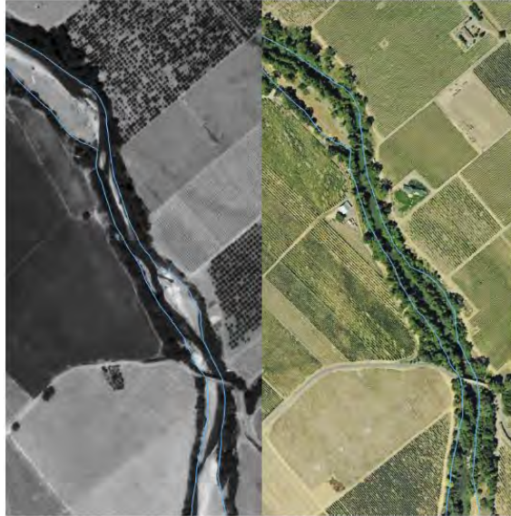
Figure 17. Example of vegetative narrowing of channel corridor near Lambert Bridge (river mile 6.6). Lambert Bridge is seen at lower right of each frame. Dry Creek flow is from top to bottom. Left frame is from 1976, right frame is from 2004. Light blue line is estimated limit of active fluvial features in 1976.
