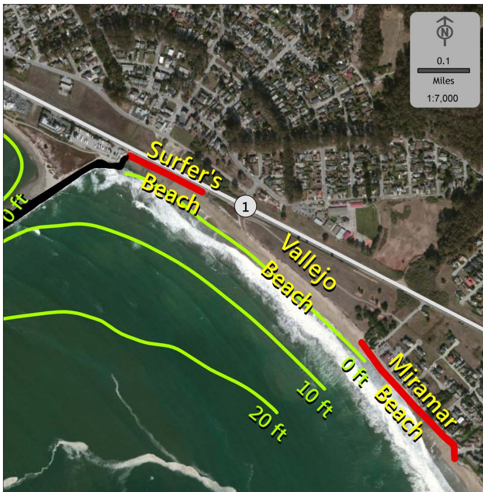
Figure 3: Local beaches, root of the East Breakwater (black line), and revetments (red lines) Contour depths are relative to MLLW.
