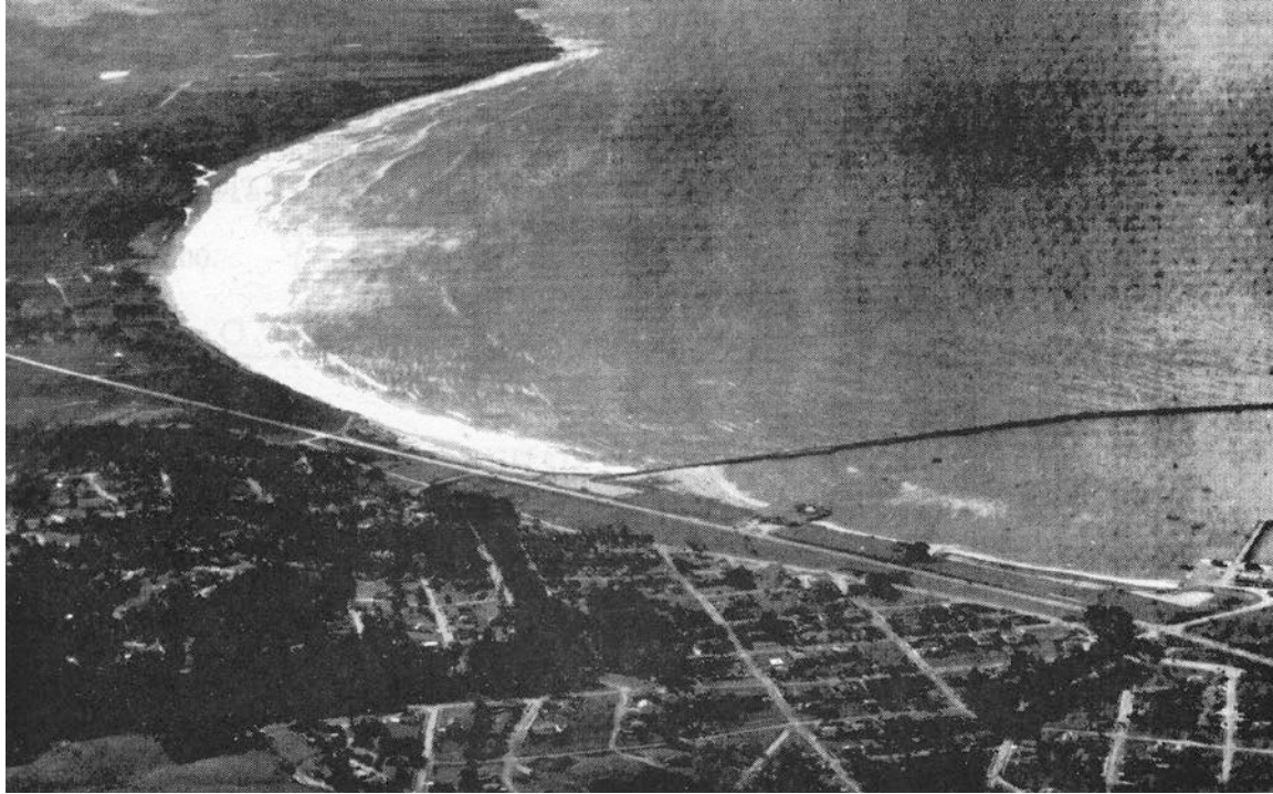
Figure 4: 1971 aerial photograph of Half Moon Bay looking south with the East Breakwater in the foreground and Miramontes Point in the distance. Note the sand wedge adjacent to the harbor side of the root of the East Breakwater. Photograph by N. Prime, USGS.
