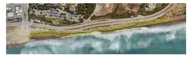
Figure 10. Approximate Footprint of Fill. Extends Approximately 3,000 Feet Along Shoreline.
