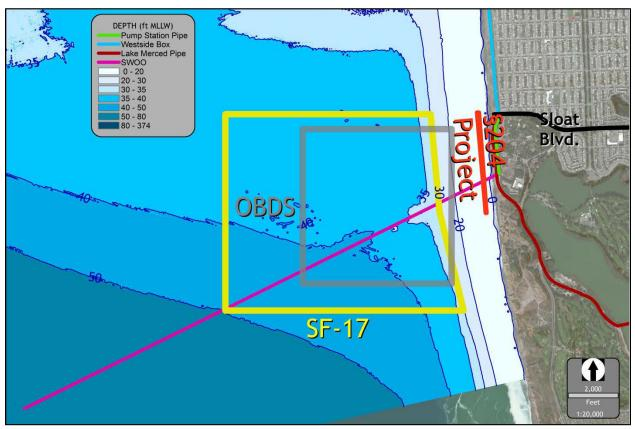
**Figure 3: Ocean Beach Demonstration Site-** Location of the §204 storm damage reduction project relative to the wastewater infrastructure (Westside Transport Box (WST), Lake Merced Water Treatment Tunnel (LMWT), and Southwest Ocean Outfall (SWOO), Ocean Beach Demonstration Site (OBDS), and SF-17). The Great Highway runs above the WST and LMWT.
