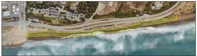
Figure 8. Approximate Footprint of Fill. Extends Approximately 3,000 Ft Along Shoreline.
