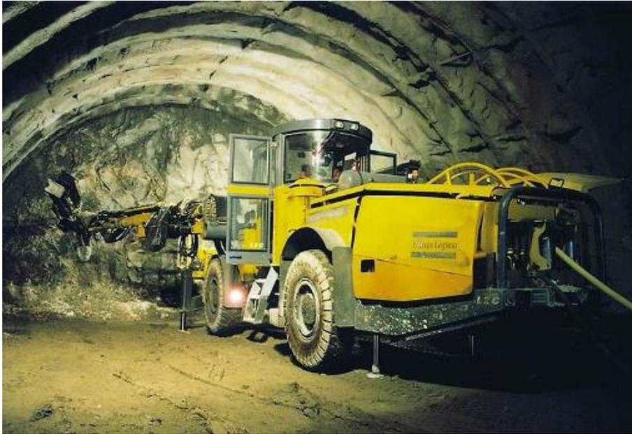
**Figure 2.7-5 Drill Jumbo for Drilling Holes**
