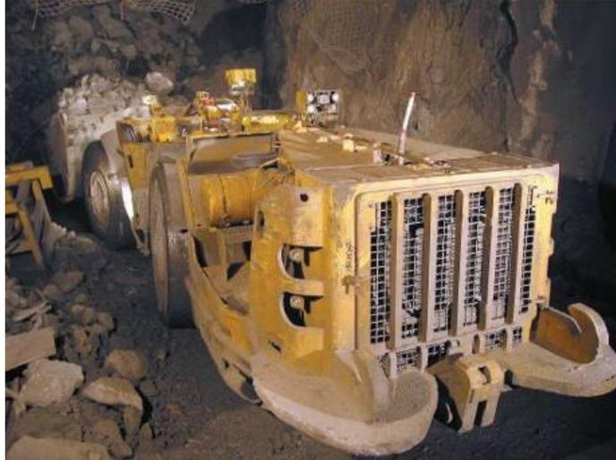
**Figure 2.7-4 Load, Haul, Dump (LHD) Unit**
