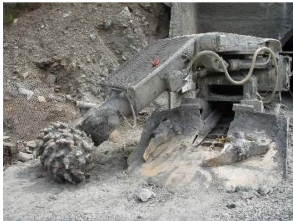
**Figure 2.7-2 Typical Roadheader Used for Tunnel Excavation in Soft to Medium Strength Rock**
