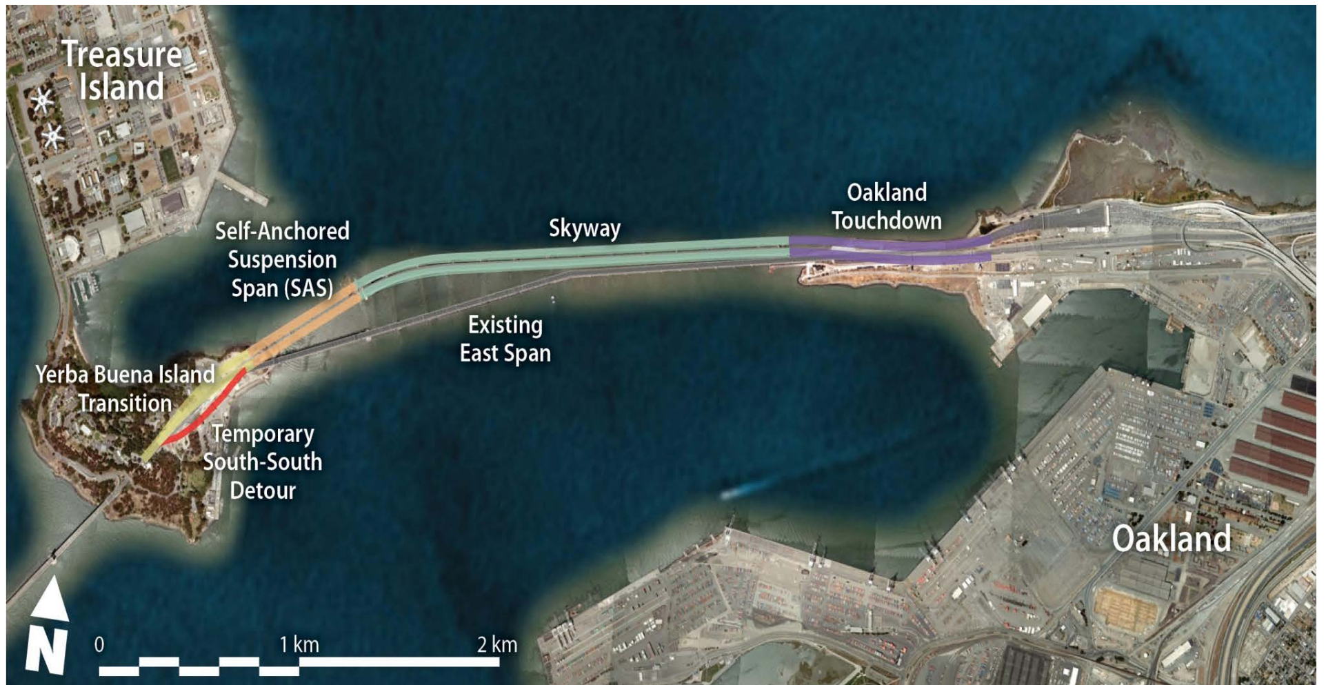
Figure 1. SFOBB East Span Seismic Safety Project map
