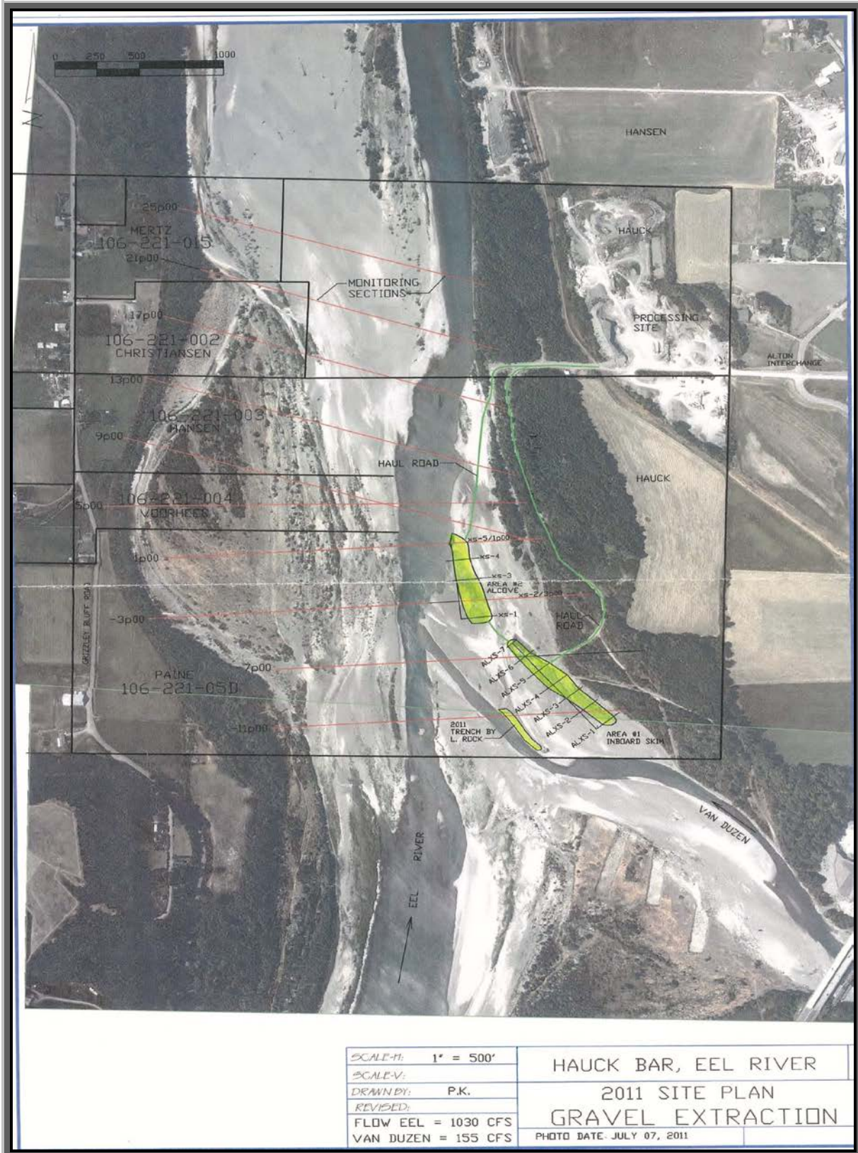
FIGURE 2: Example pre-extraction aerial photo w/ extraction zone cross sections delineated.
