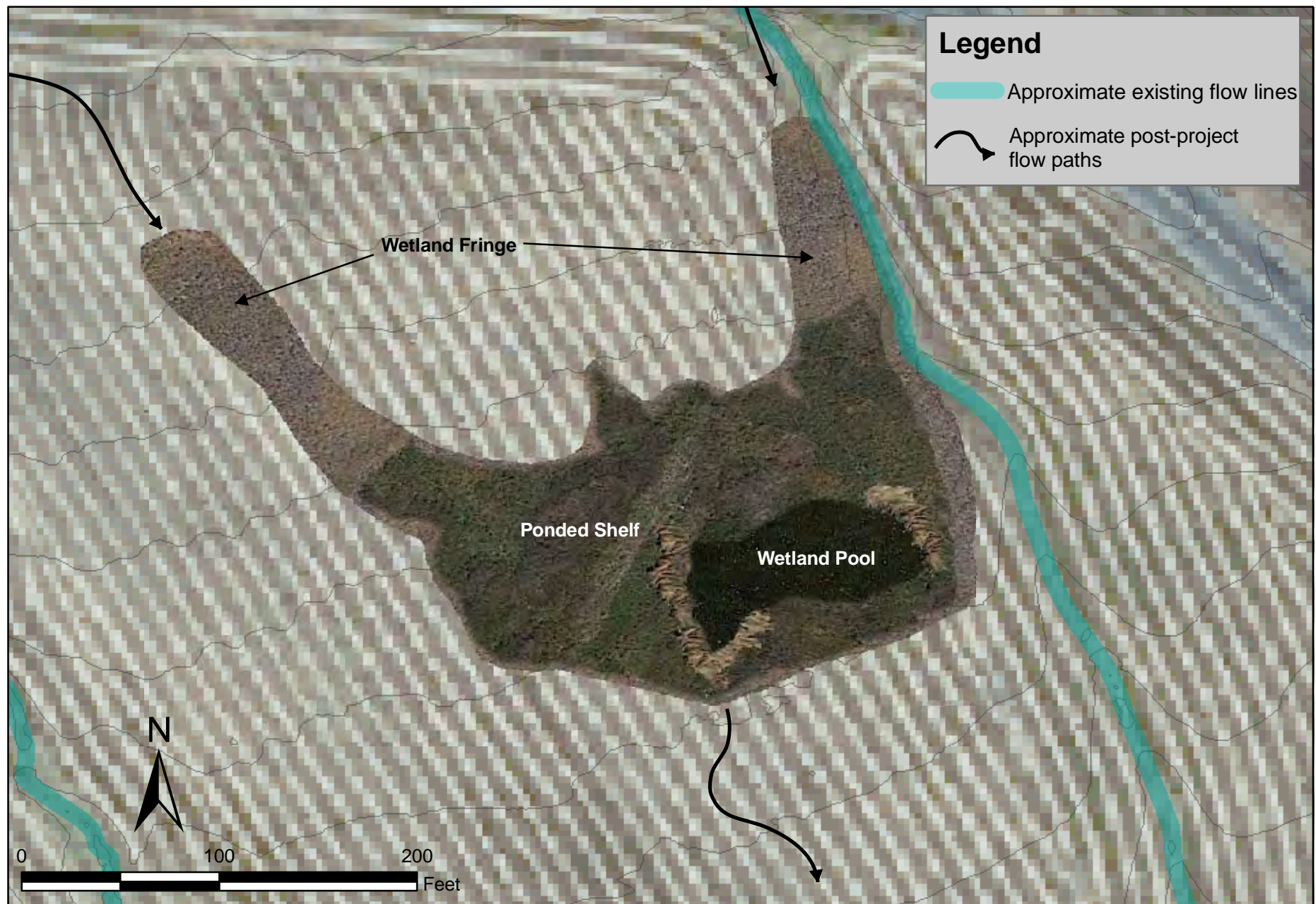
Figure 2. Conceptual plan for Wetland 2, Cayetano Wetland Preserve near Livermore, Contra Costa County, California. Plan shows approximate extent of the deep portion of the pool, the shallow ponded area (ponded shelf), and the saturated wetland fringe area. See Figures 3 and 4 for conceptual cross-sections of this feature.
