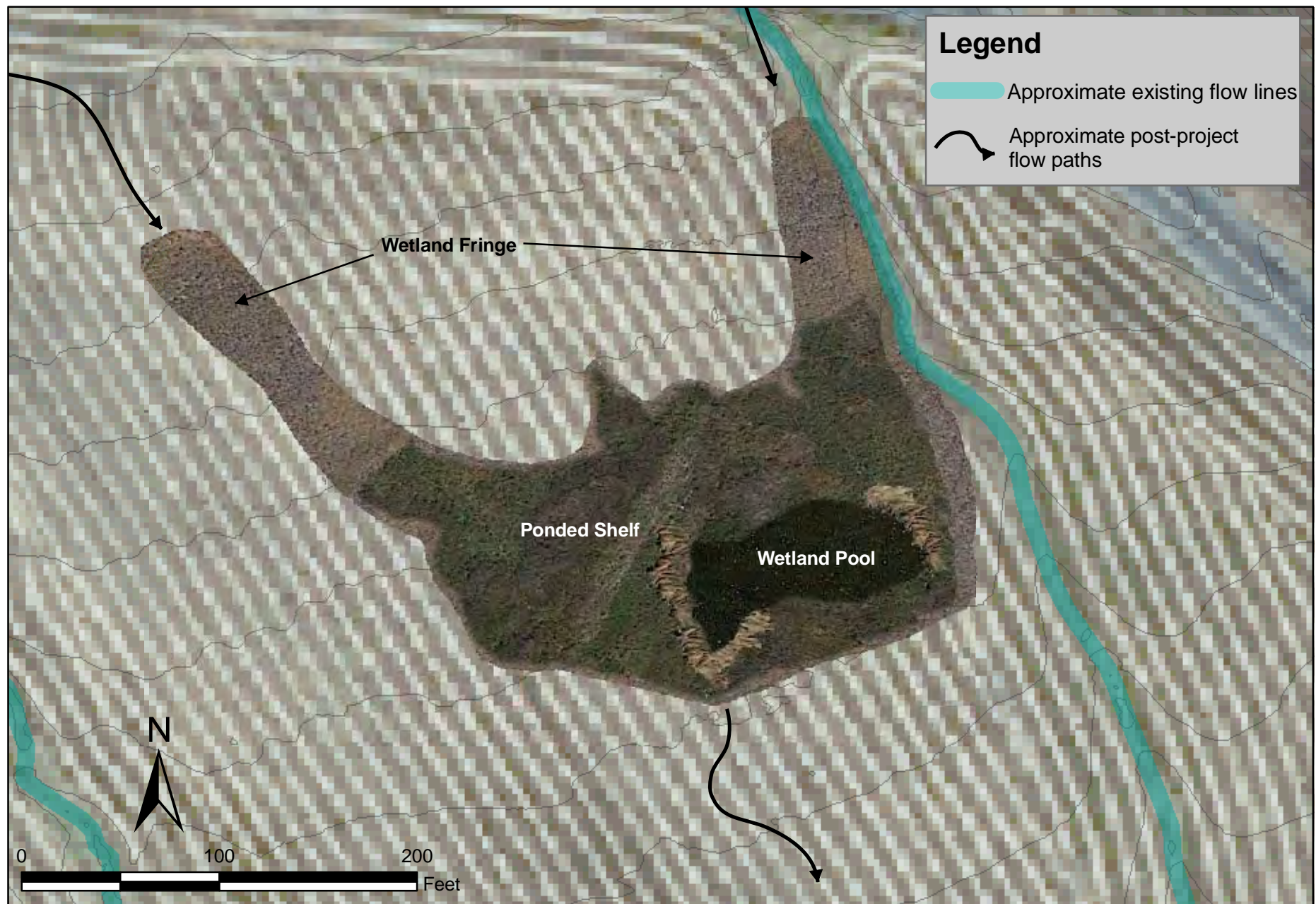
Figure 3. Conceptual plan for Wetland 2, Cayetano Wetland Preserve near Livermore, Contra Costa County, California. Plan shows approximate extent of the deep portion of the pool, the shallow ponded area (ponded shelf), and the saturated wetland fringe area.
