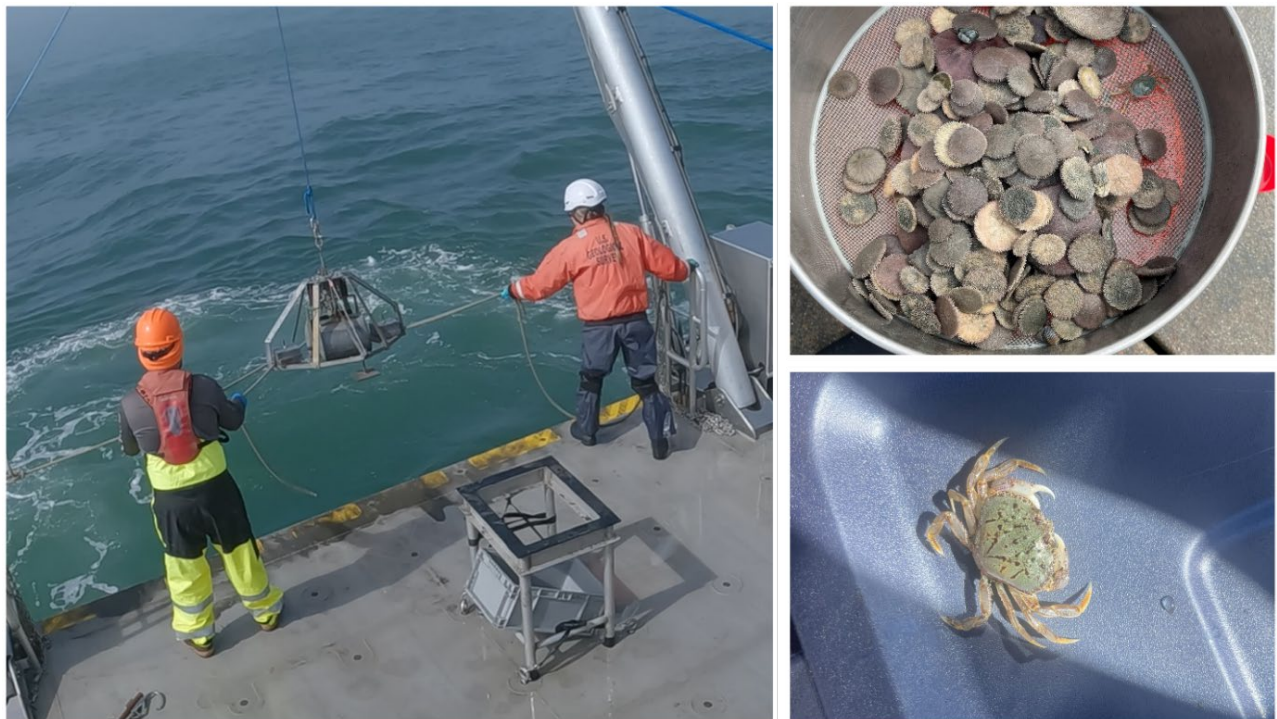
Figure 2. Benthic Samples collected using a Smith-Mac Grab from the USGS R/V Parke Snavelly and Cal Poly Humboldt R/V North Wind.
