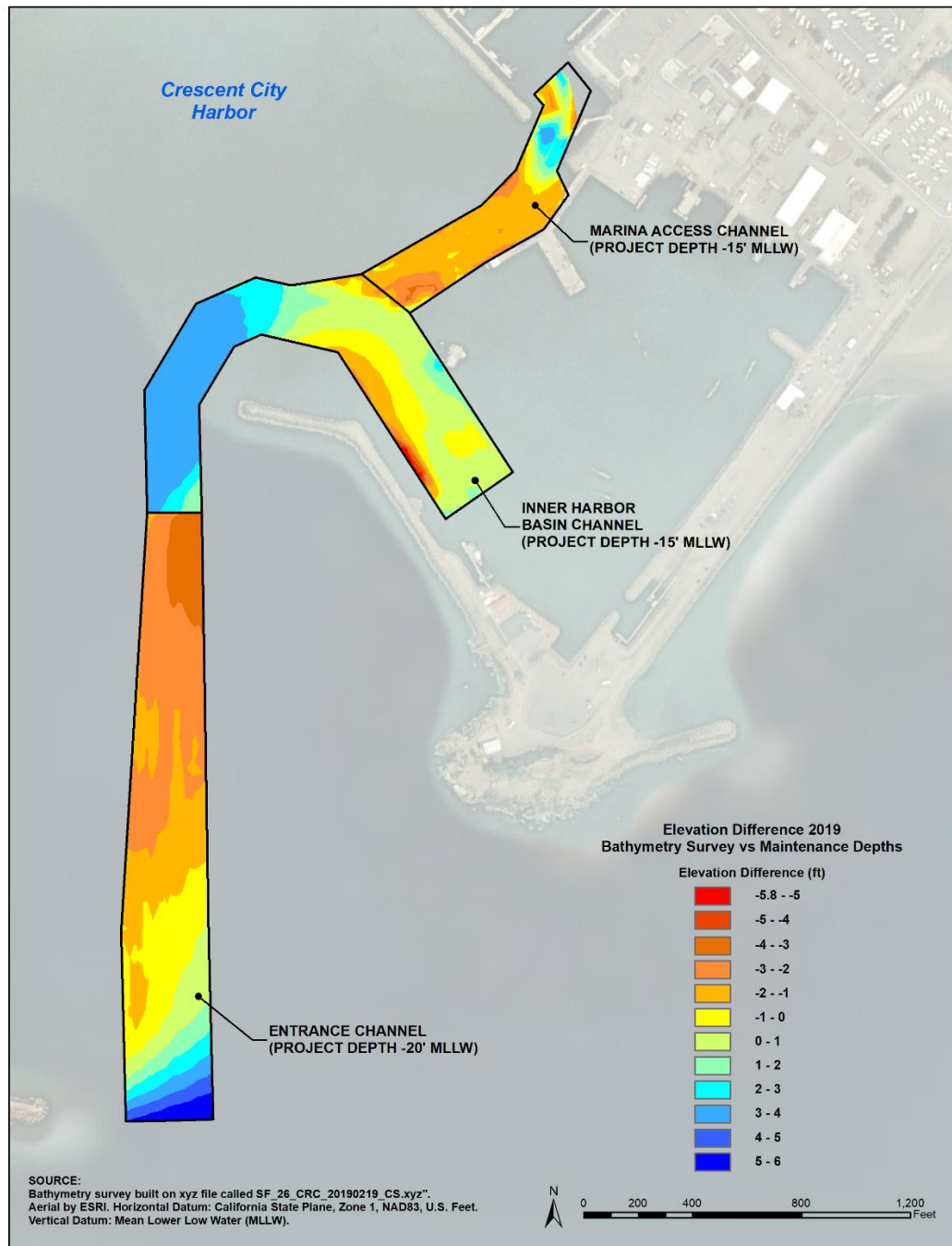
Figure 2. Crescent City Harbor Federal Channel Dredging Footprint Based on 2019 Hydrographic Surveys
