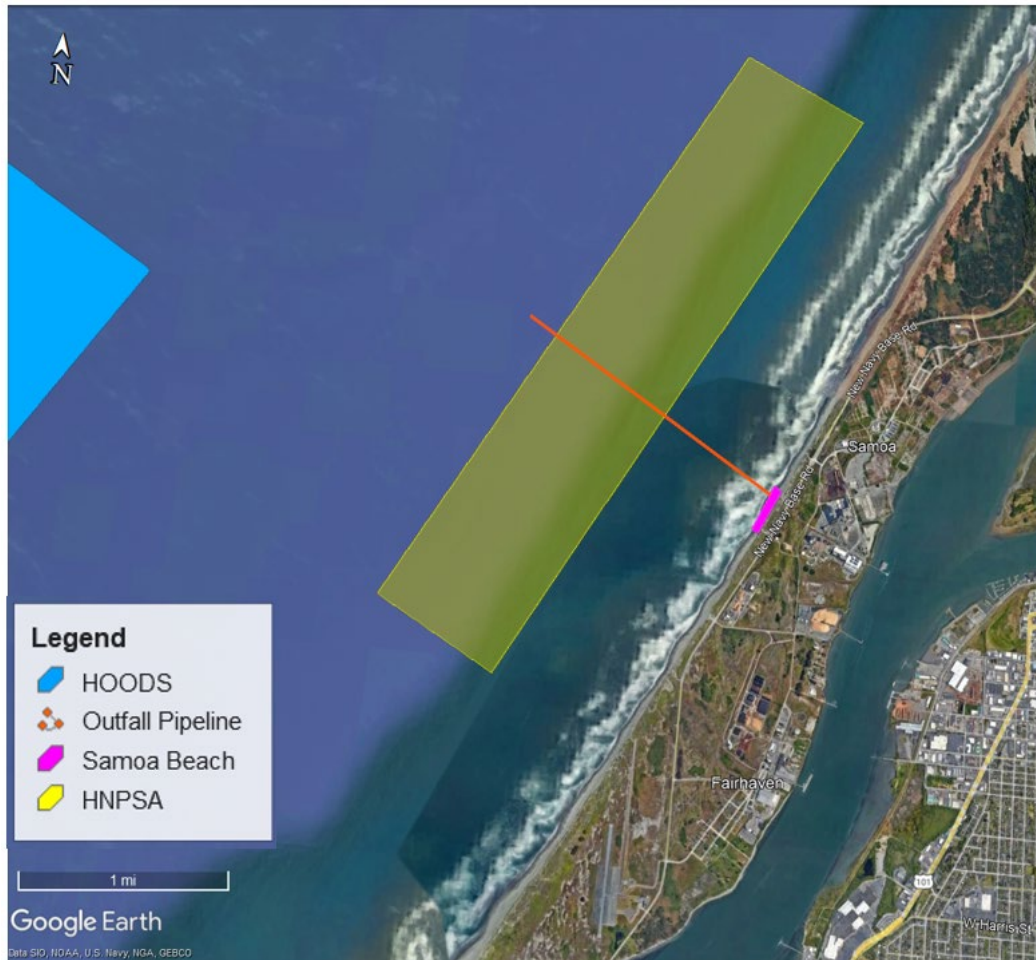
Figure 9. Outfall pipeline location in relation to HNPSSA and HOODS. Note, pipeline only exposed after severe erosional events. Emergency temporary measures have been taken to cover the pipeline, highlighting the ongoing need for sediment management in this area
