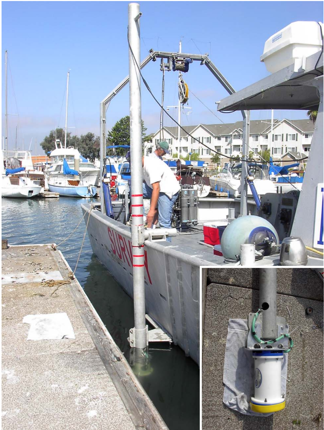
Figure 2. Side mounting location of ADCP.
