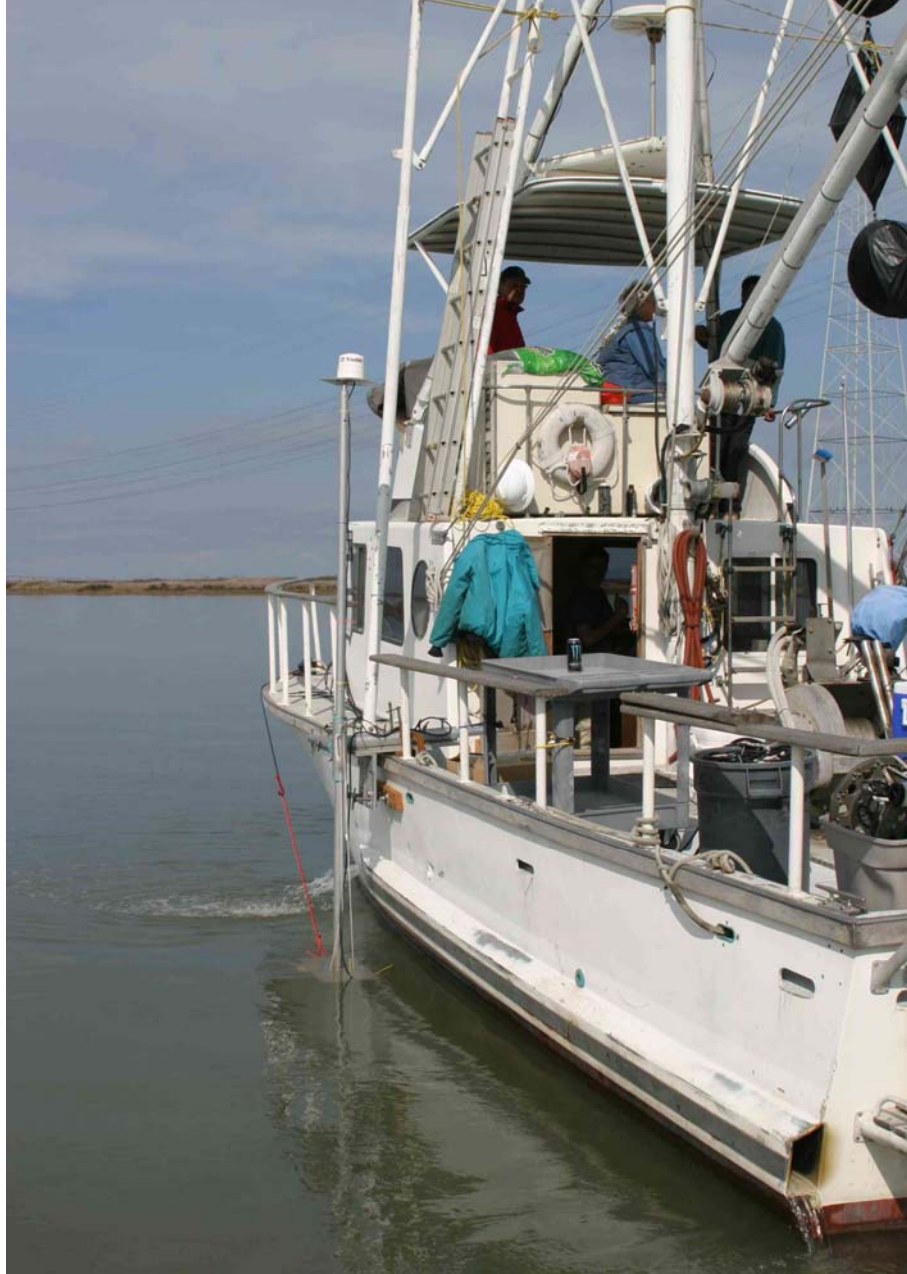
Figure 6. Survey vessel R/V Shearwater, showing ADCP-integrated DGPS mounted on the port side with transducer assembly riding just below the surface of the water.
