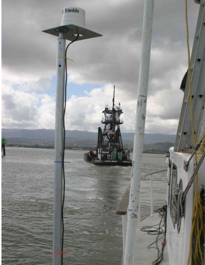
Figure 9. Running a parallel ADCP transect directly behind the knockdown barge.
