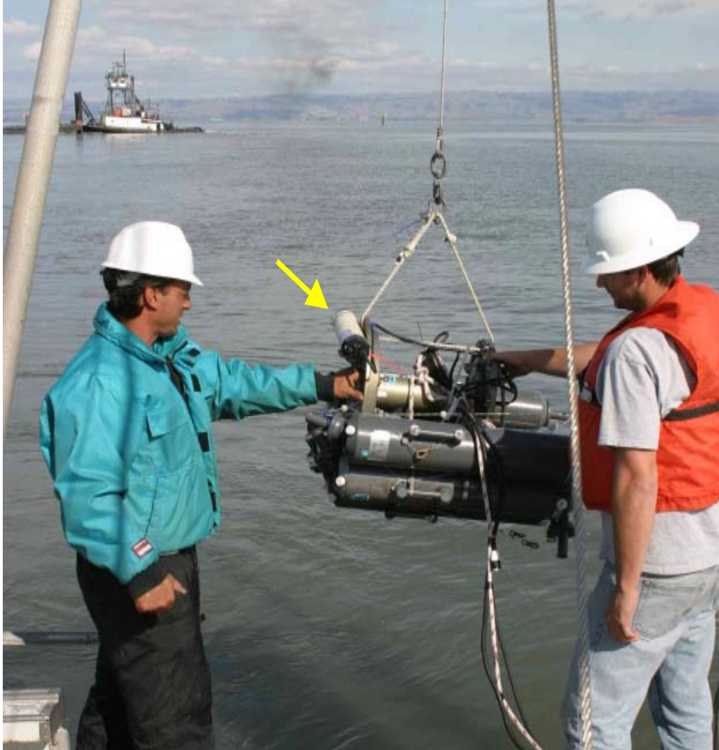
Figure 11. Modified rosette water sampler with OBS unit attached (indicated by arrow).
