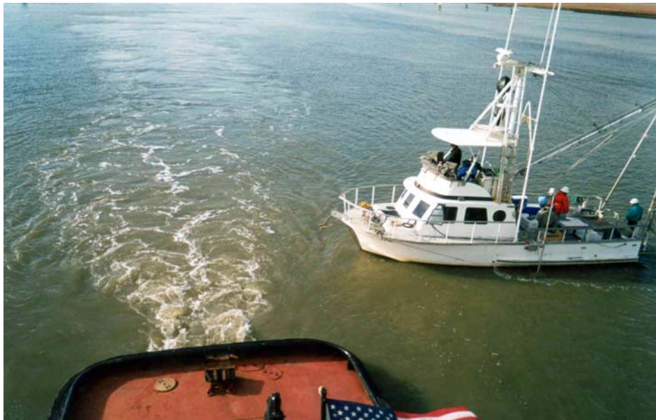
Figure 10. Running a perpendicular ADCP transect behind the stern of the tug pushing the knockdown barge.
