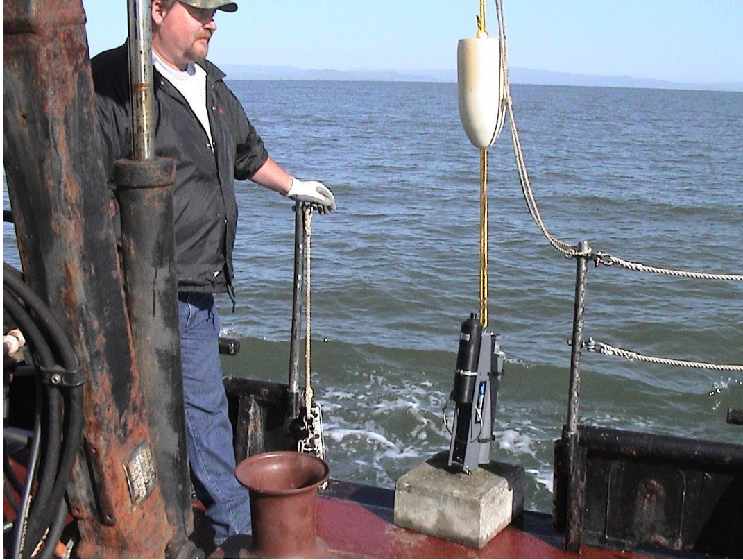
Fig. 5 Mooring configuration with acoustic release used at sites throughout the study area in 2007-8
