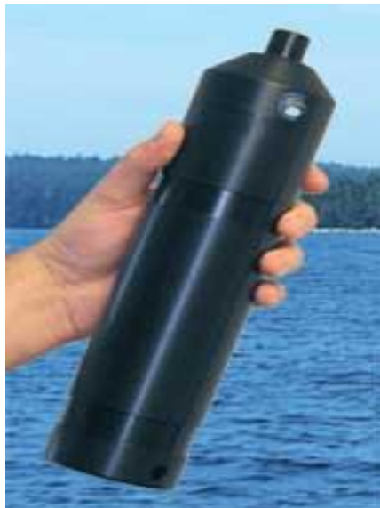
Fig. 2. Automated, tag-detecting receiver (VEMCO VR2).
