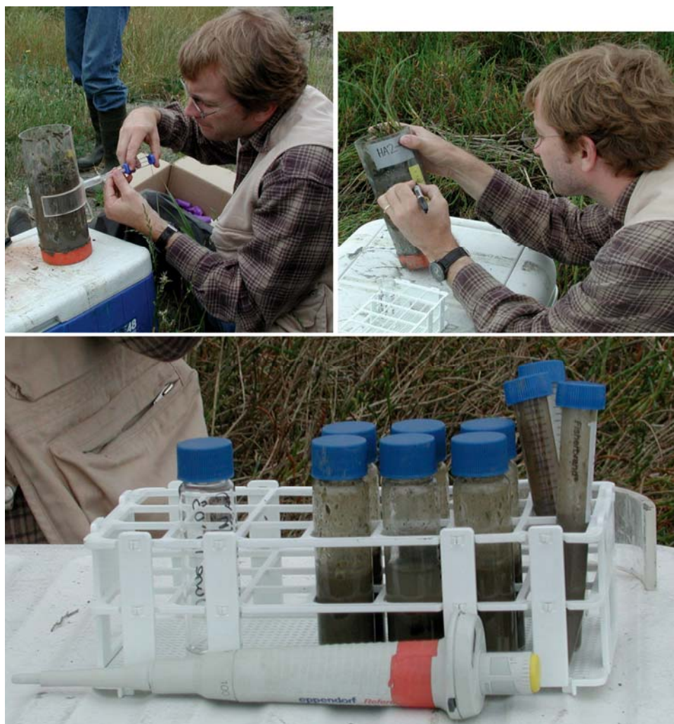
Figure 3-3. Administering isotopes to sediment cores and epipelon suspensions
