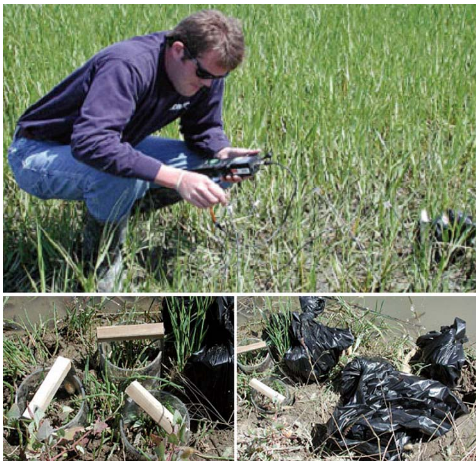
Figure 3-4. Incubation of vegetated cores in light and in darkness (upper); and onsite determinations of redox potential and pH (lower)
