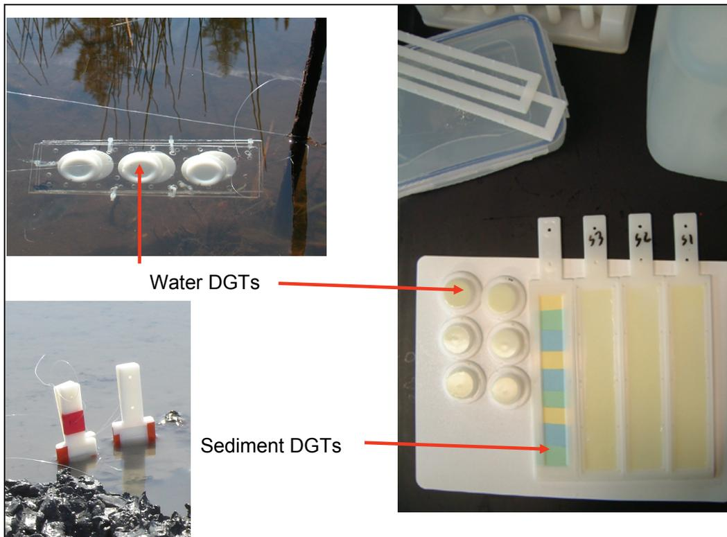
Figure 2. Water and sediment DGTs were deployed on the sites located in San Pablo Bay and South San Francisco Bay (CA) and sampled after 3, 14, and 28 days of exposure to site conditions.
