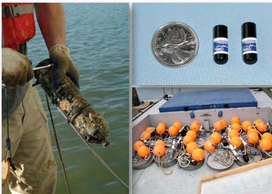
**Figure 5.** Underwater ultrasonic receiver (left), Vemco V7 and V9 tags (upper right), and deployment riggings with acoustic releases for deepwater deployment of receivers in San Francisco Bay (lower right).
