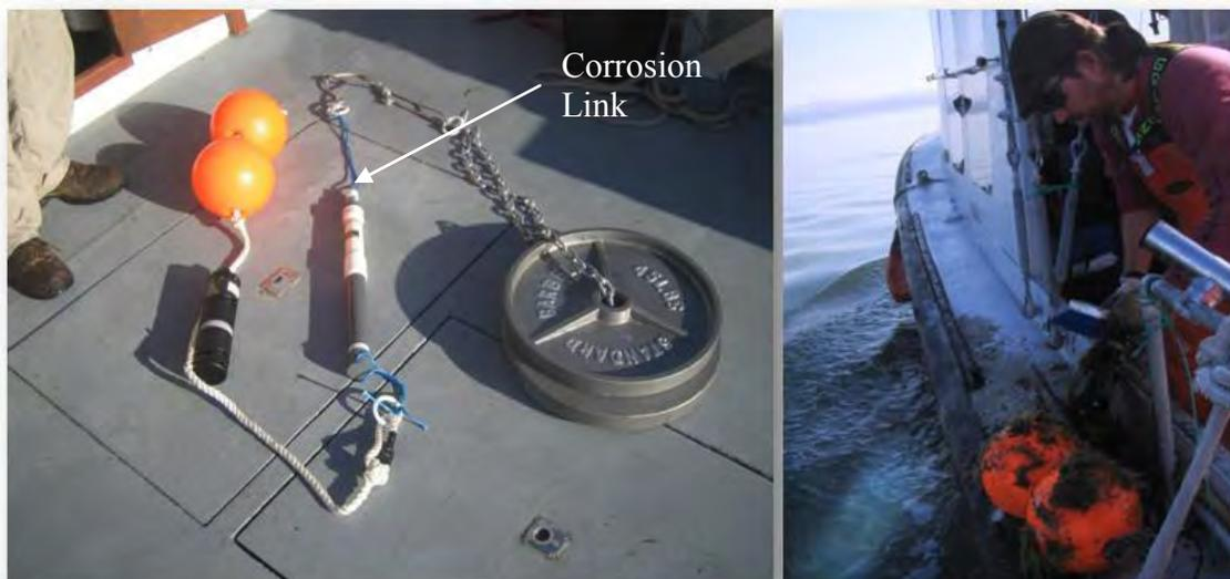
**Figure 9.** Left: VR2/VR2W ultrasonic receiver rigging with acoustic release, attached to steel weights (Photo: Alex Hearn). Right: Retrieval of receiver – the buoys float to the surface with the receiver and acoustic release still attached. (Photo: Michele Buckhorn).
