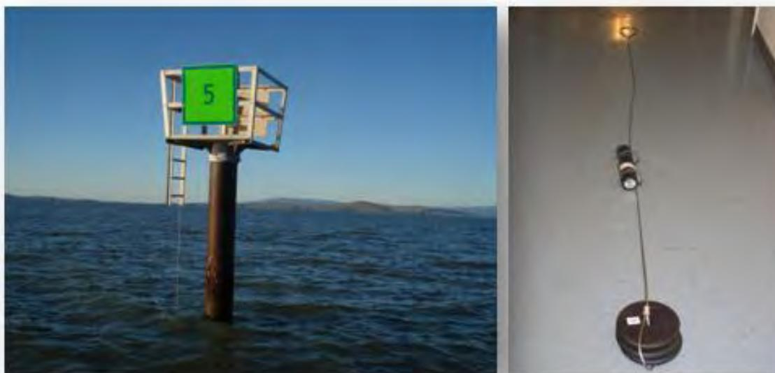
**Figure 8.** Left: VR2/VR2W ultrasonic receiver rigging from a channel marker in San Pablo Bay Right: VR2W mooring design for fixed stations (Photos: Eric Chapman).
