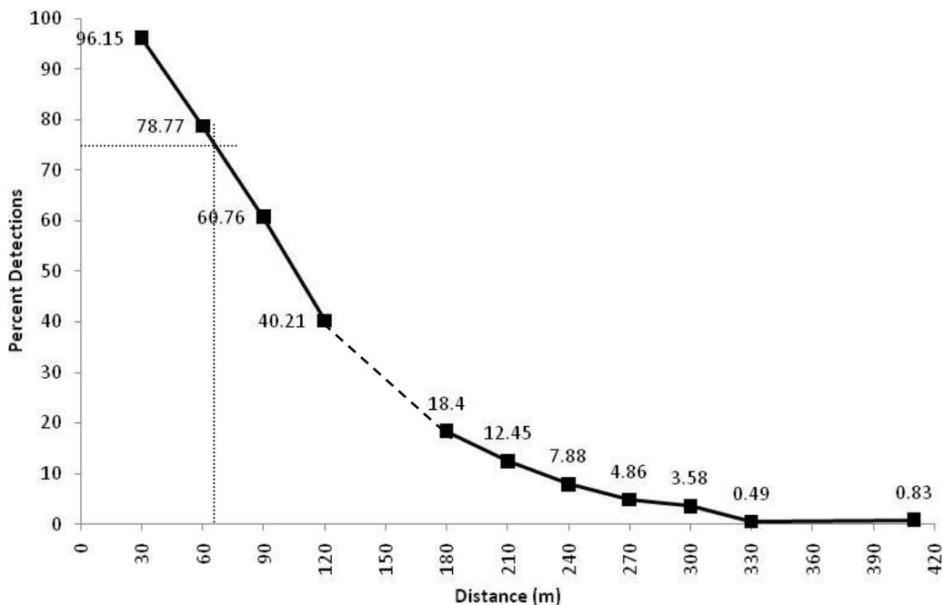
Figure 11. Detection efficiency of VR2W receivers during range tests in San Pablo Bay, November 2008.
