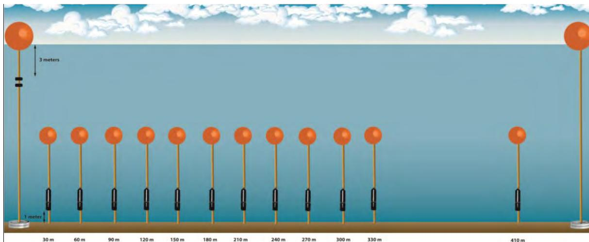
**Figure 10.** Range test experimental design at SF10 placement site. Receivers are attached to moorings that are weighted down with 4 x 10 lb. weight plates. Receivers are spaced every 30 meters up to 330 meters and then a last receiver at 410 meters. Not to scale.
