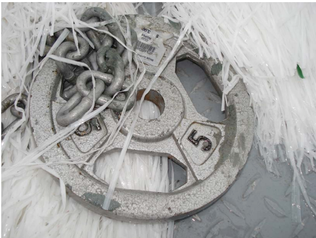
Figure 2-4. Transect 1: Evidence of Weighted Tails Reaching Surficial Sediment
