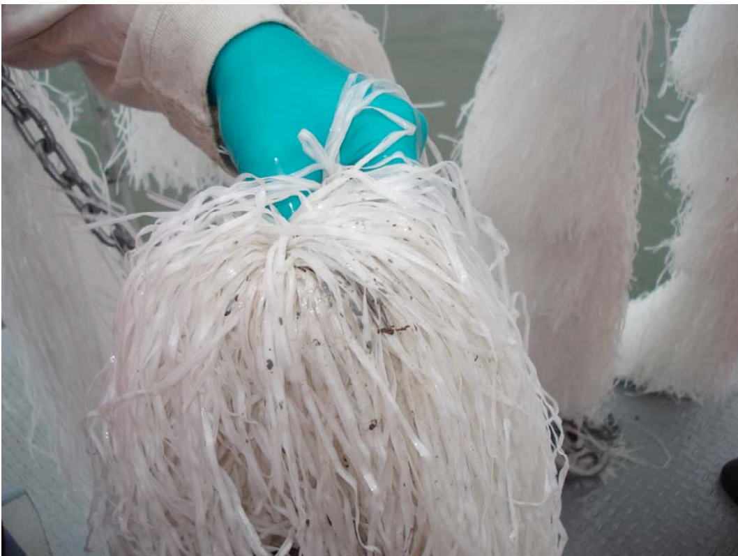
Figure 2-6. Transect 1: Presence of Material Retained on Oil Snare
