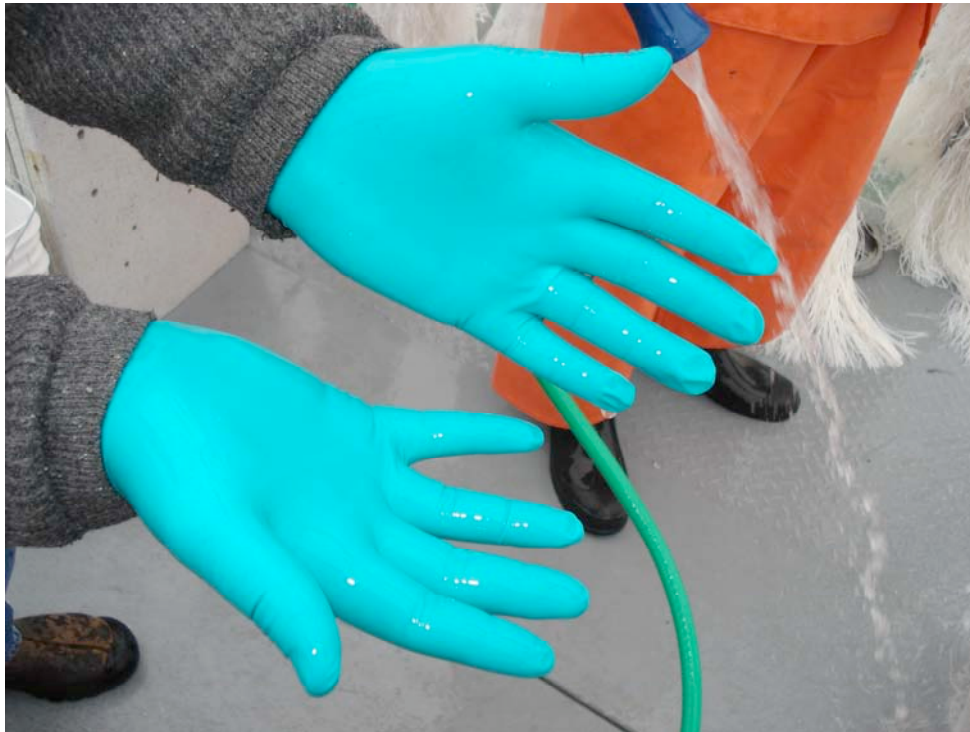
Figure 2-17. Transect 2: Material Easily Washed Off of Nitrile Gloves – No Petroleum Retained
