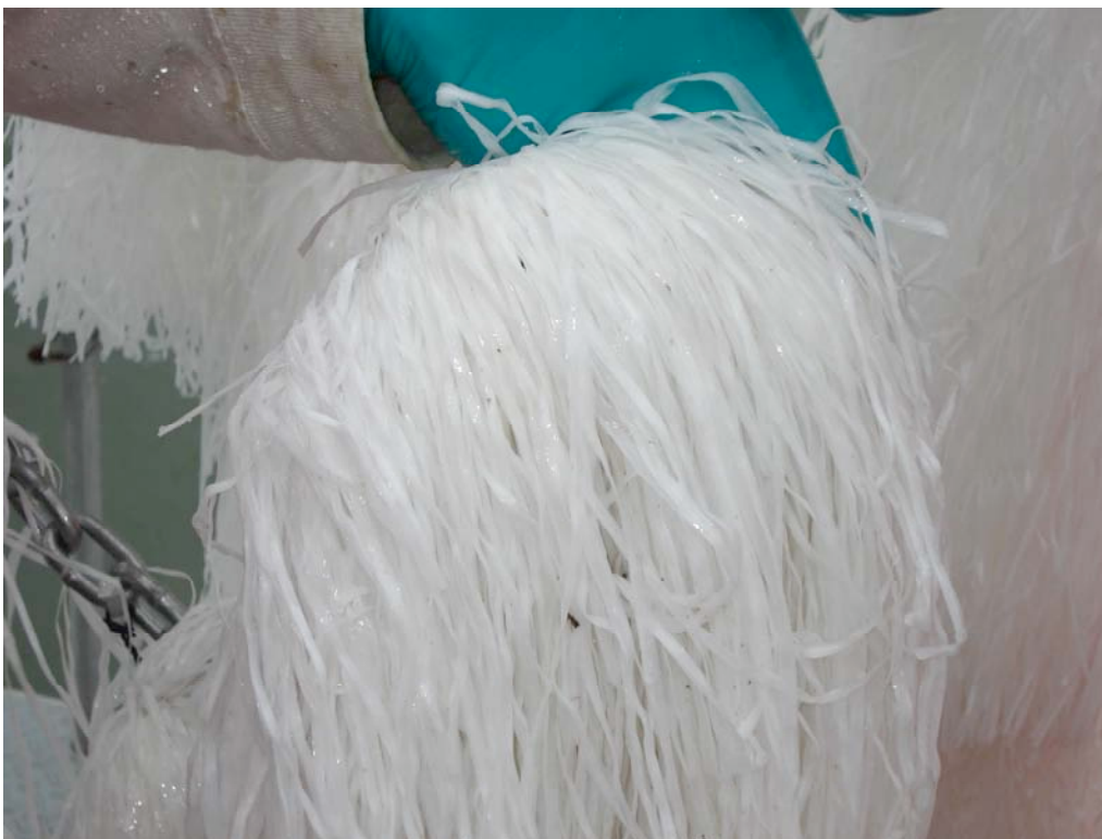
Figure 2-10. Transect 1: Verification that Oil Snare Did Not Retain Any Petroleum Product
