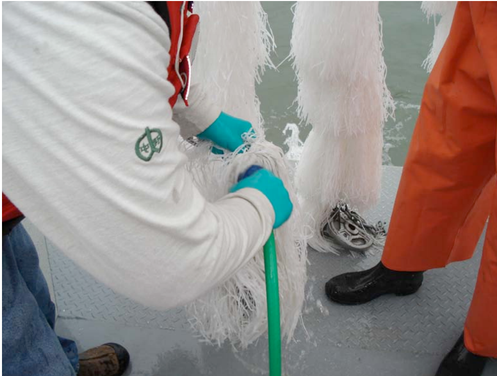
Figure 2-9. Transect 1: Rinsing of Oil Snare Apparatus with Site Water
