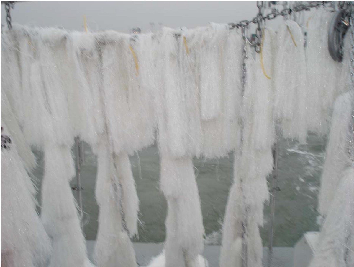
Figure 2-19. Transect 2: Verification that Oil Snare Did Not Retain Any Petroleum Product
