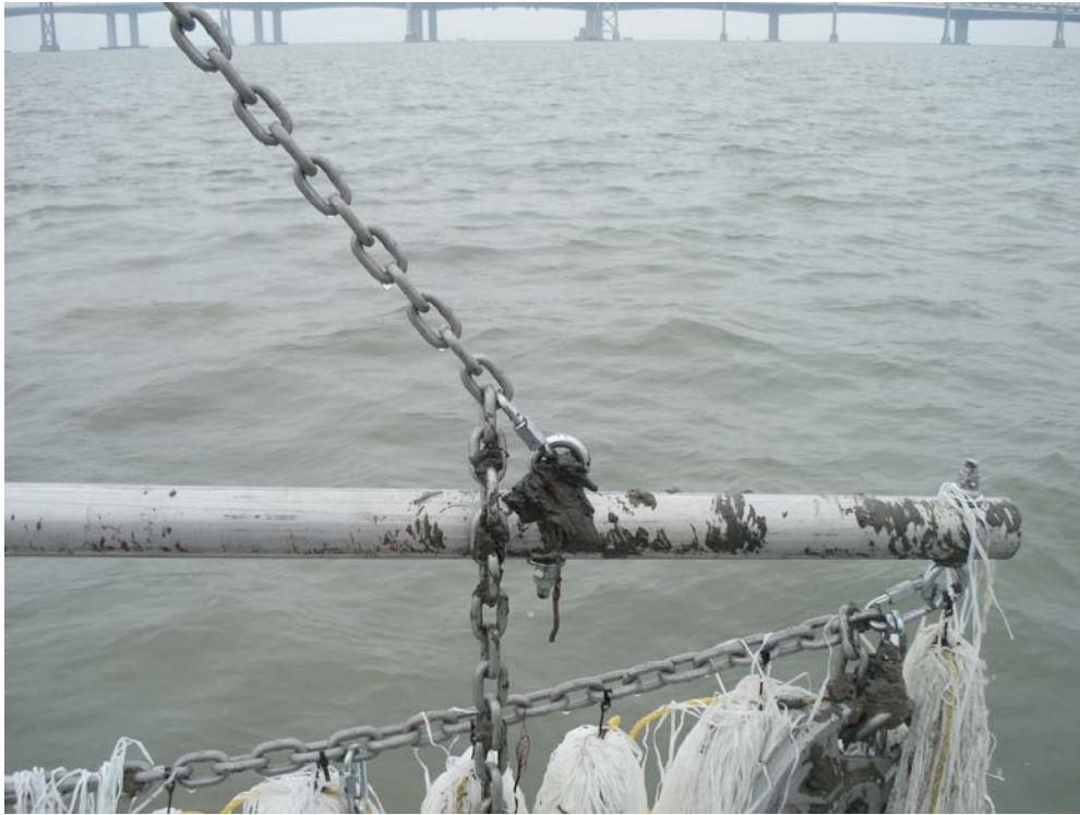
Figure 2-13. Transect 2: Evidence of Beam Reaching Surficial Sediment
