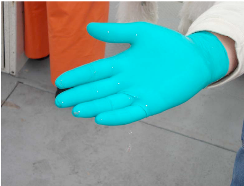
Figure 2-8. Transect 1: Material Easily Washed Off of Nitrile Gloves – No Petroleum Retained
