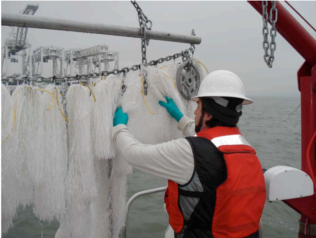
Figure 2-5. Transect 1: Inspection of Oil Snares
