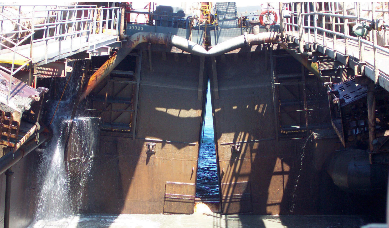
The Essayons releasing sediment suitable for unconfined aquatic disposal via its split hull.
