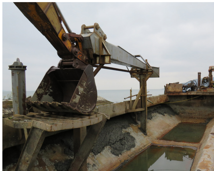
There are four different types of dredge heads, these are shown above and on the following page. Dredge heads include clamshell ( left ) and excavator/dipper ( right ).
