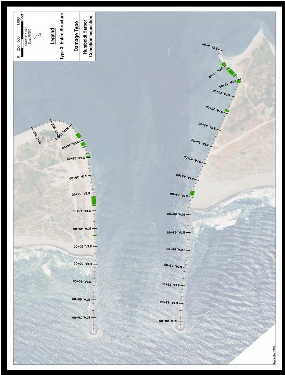
**Figure 4: Repair type and locations**
