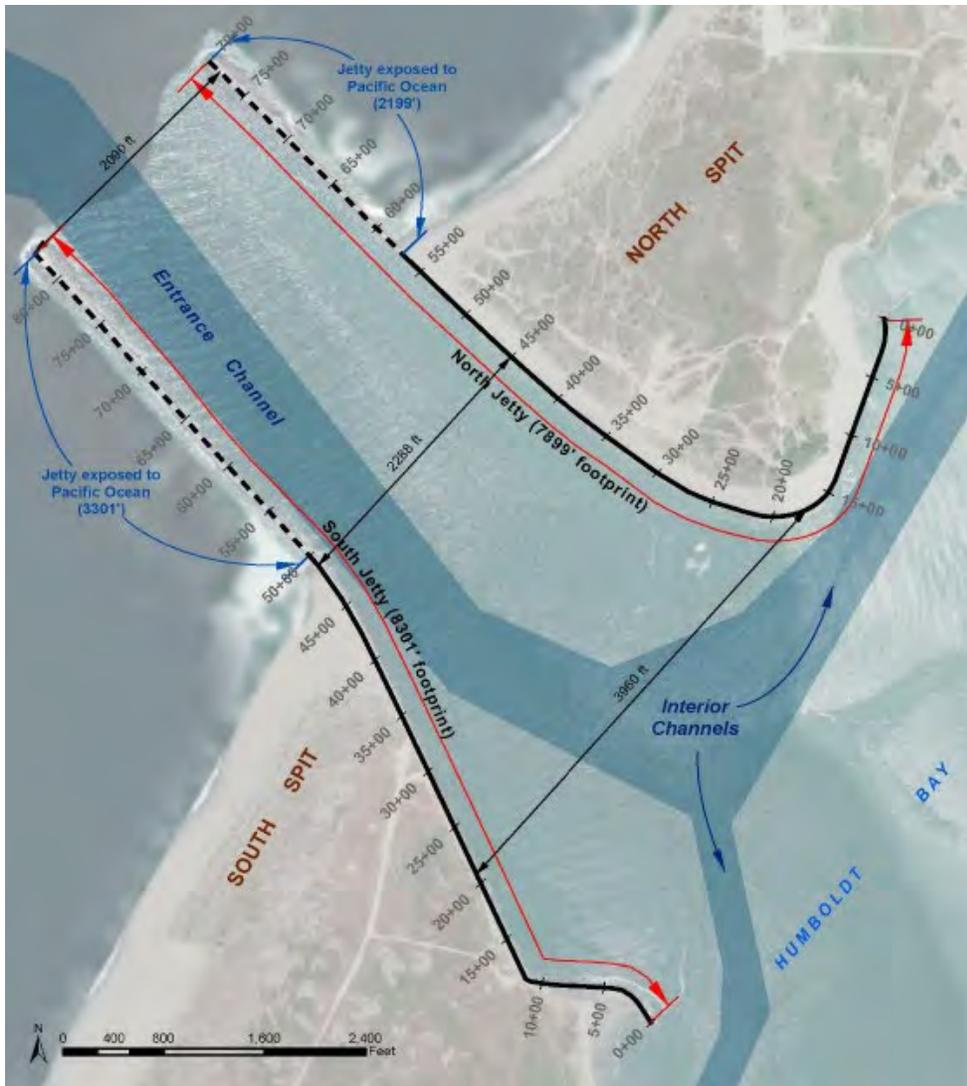
Figure 2. US Army Corps of Engineers map of harbor entrance and jetty stationing.
