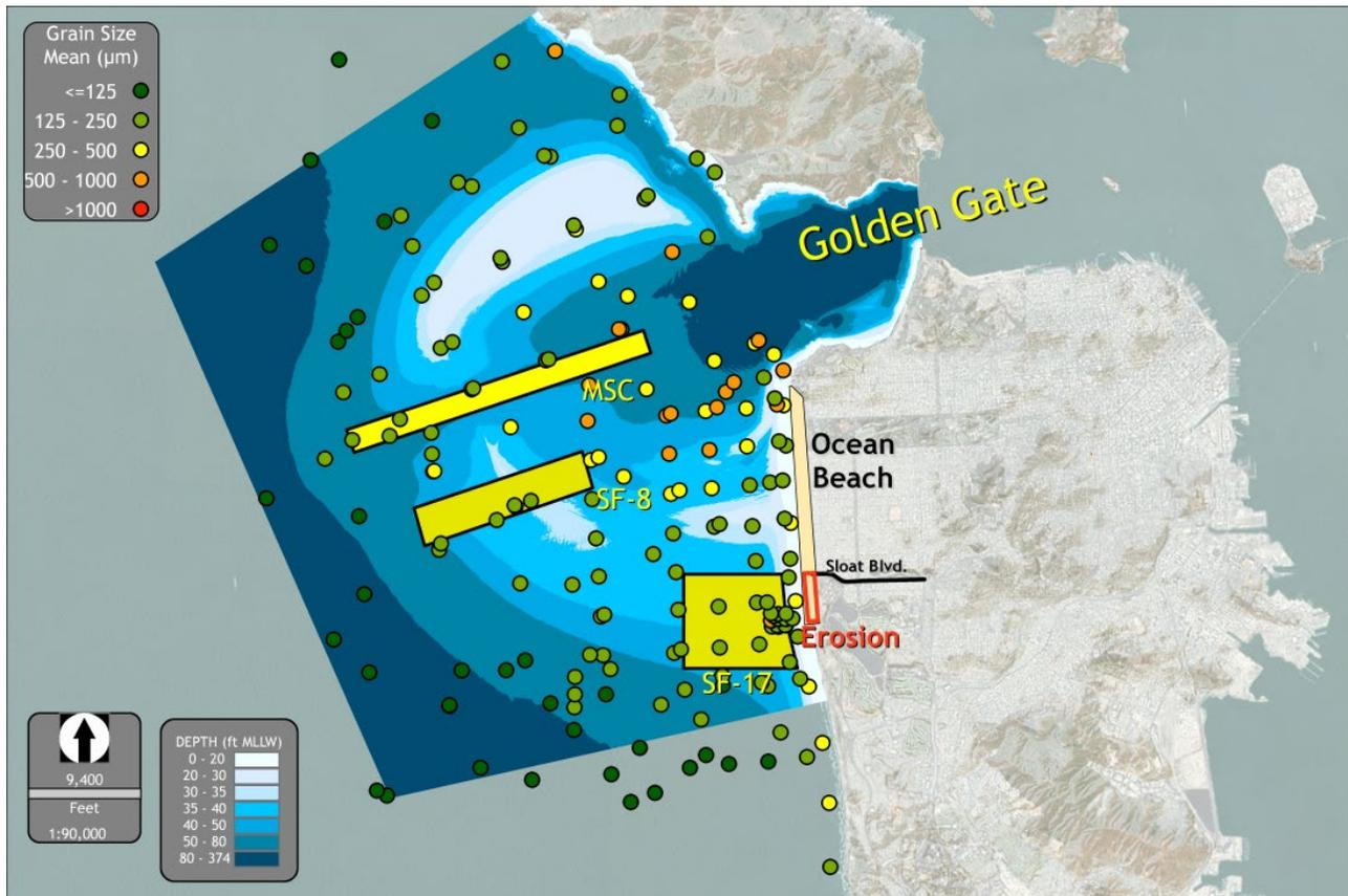
**Figure 14:** Grain-size distribution outside of the Golden Gate.
