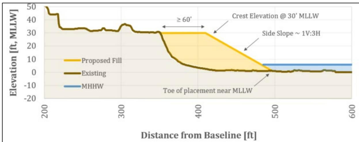
**Figure 4. Example Cross-Section 27. (Plan View location shown in Figure 7)**
