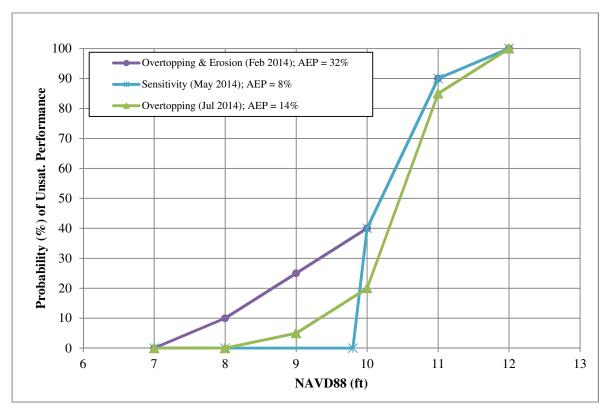
Figure 35: Outboard Dike Fragility Curves Developed.
