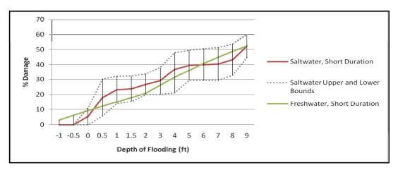
Figure 8: Structure Depth-Damage Relationship, 2-Story SFR
