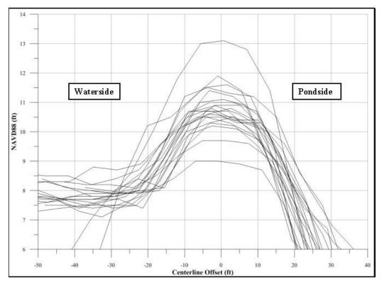
Figure 31: Cross sections along the Outboard Dike
