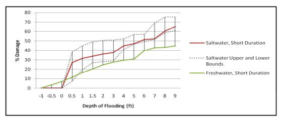
Figure 10: Structure Depth-Damage Relationship, Industrial
