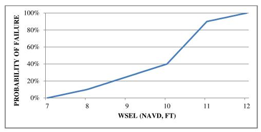
Figure 5: Input 2 - Outboard Dike Failure Function
