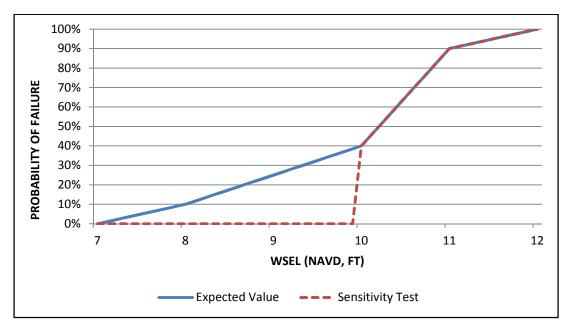
Figure 36: Levee Failure Function Comparison – Economic Justification Sensitivity Test
