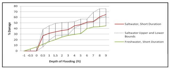
Figure 9: Structure Depth-Damage Relationship, Commercial
