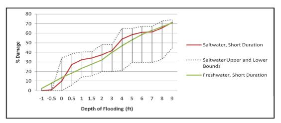
Figure 7: Structure Depth-Damage Relationship, 1-Story SFR
