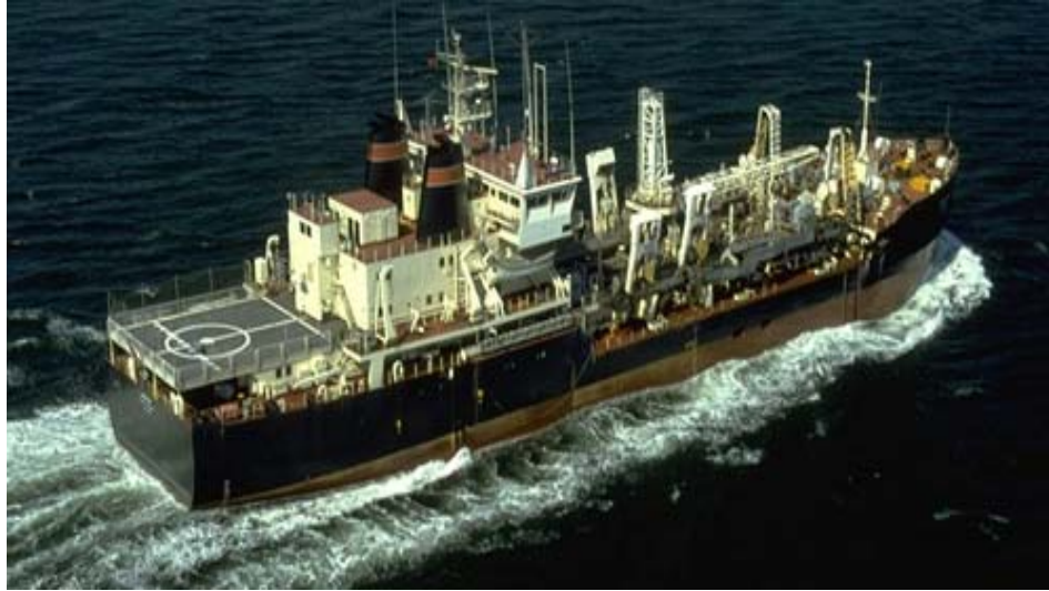
Figure 7: Hopper Dredge Essayons.
