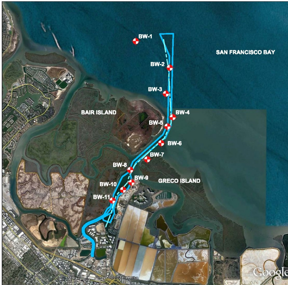
Figure 2. Plan View of Redwood City Harbor Boring Locations from Fugro Geotechnical Data Report.
