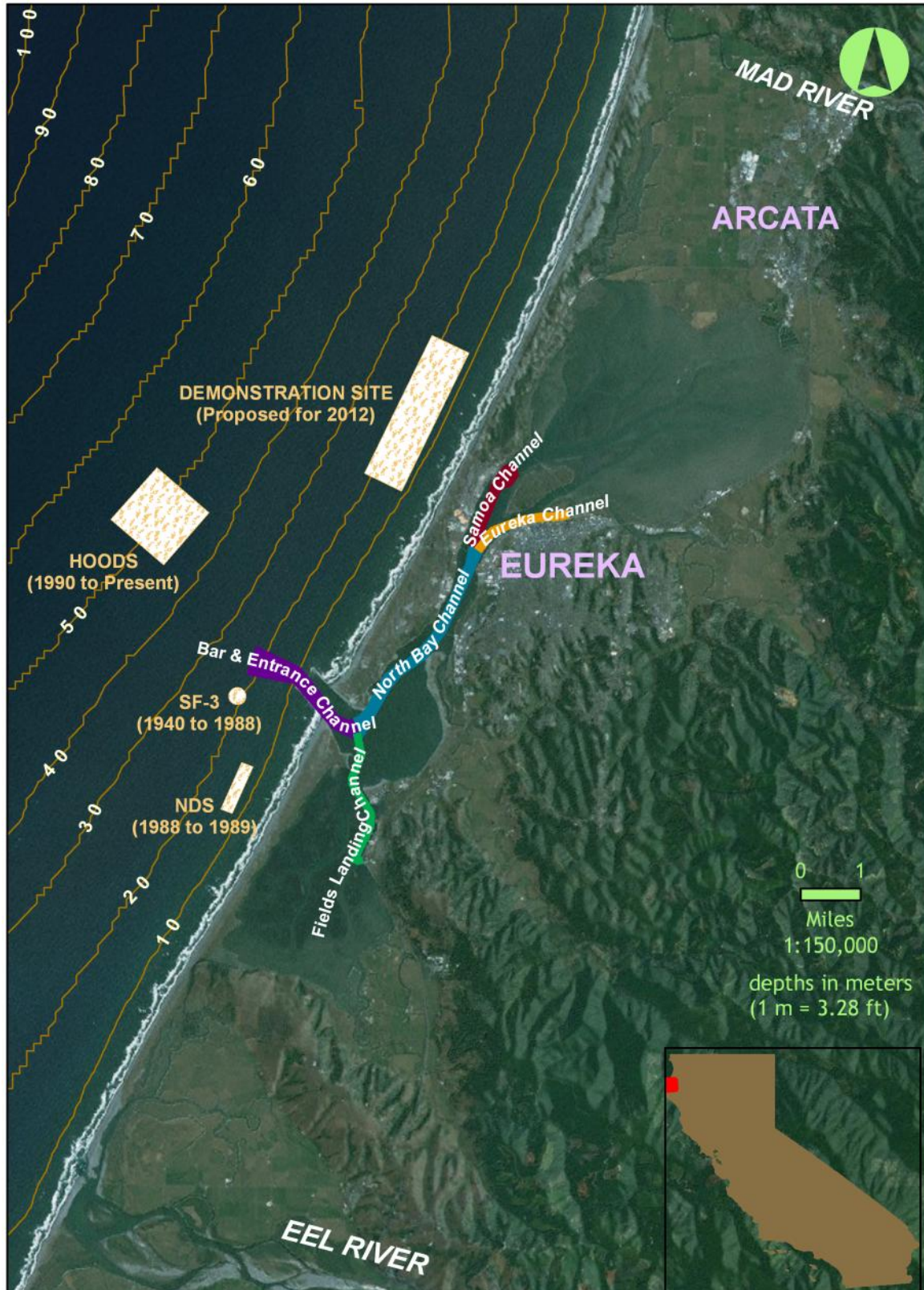
Figure 1. Humboldt Bay Dredging Channels and Placement Sites. Humboldt County, California. Datum: Mean Lower Low Water
