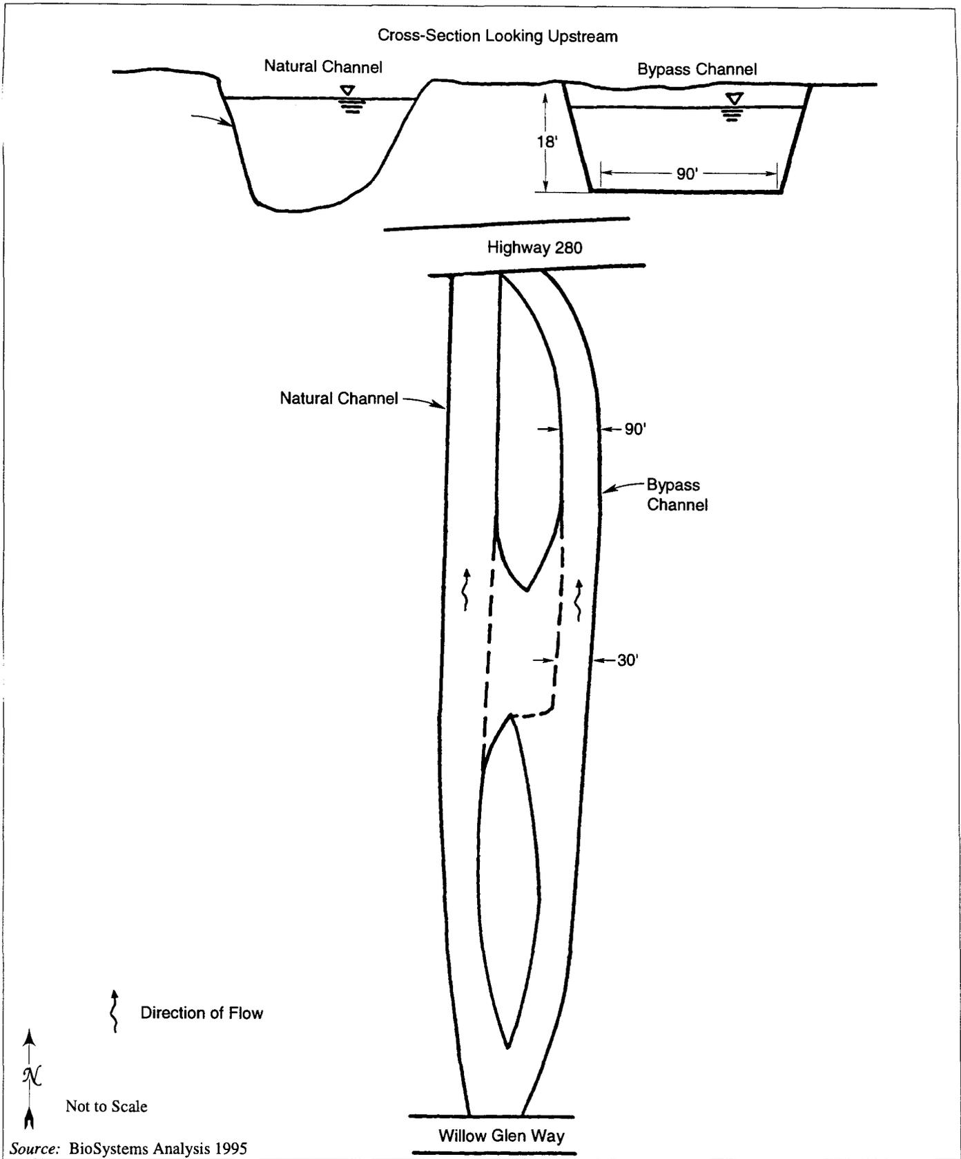
**Figure 2-5. Conceptual Earth Bypass Channel Plan Design**
