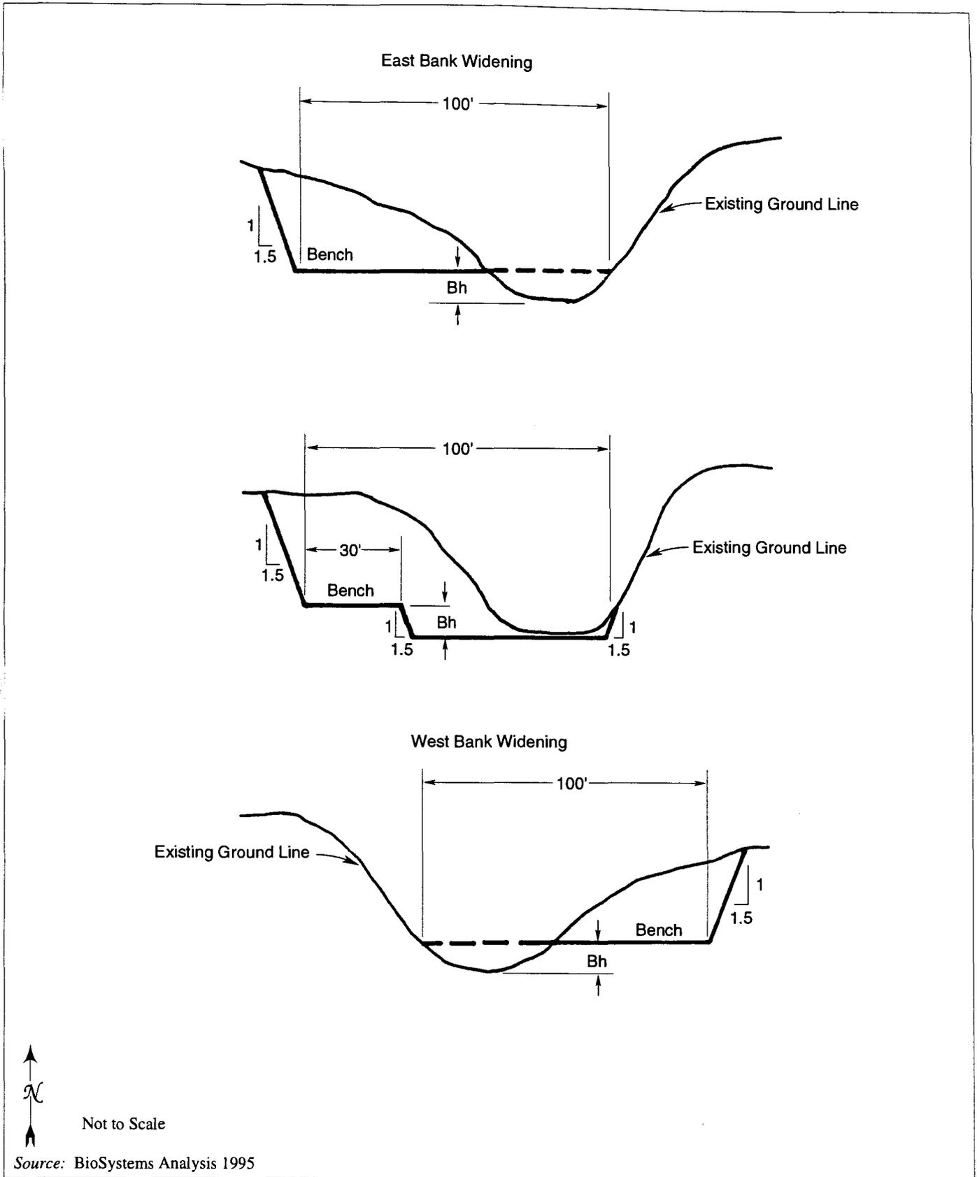
**Figure 2-4. Conceptual Widened Earth Channel Plan Designs**
