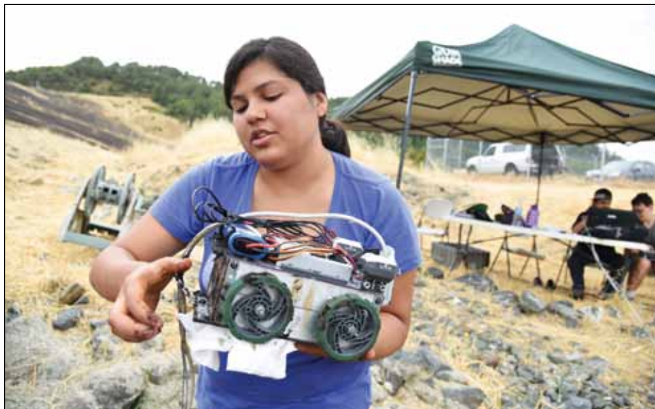
[Above] Pittsburg HS senior Catalina Vera prepares to place a robot car into a toe drain at Lake Mendocino.
